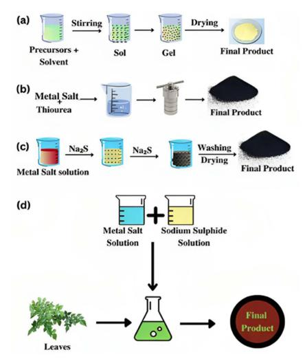
Fig. 3 Graphical depiction of the (a) sol-gel, (b) hydrothermal, (c) precipitation, and (d) green synthesis methods.<sup>10</sup>
