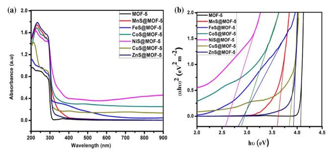
Fig. 15 (a) UV-vis spectrum (b) Tauc plot of bare MOF-5 and TMS@MO5.65
