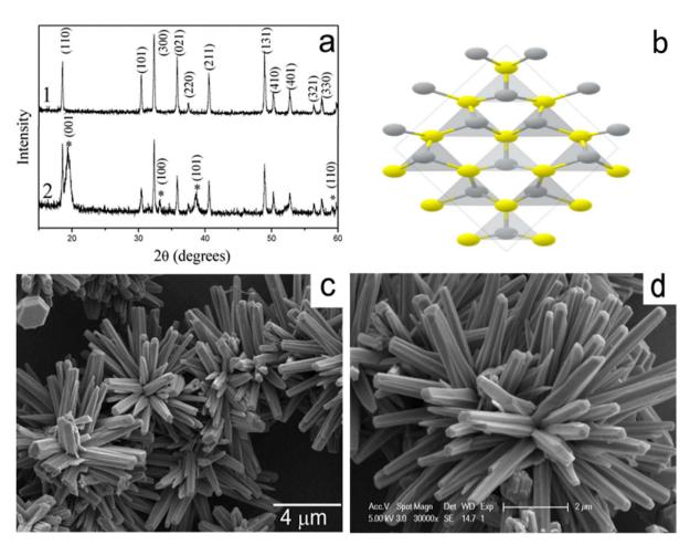
(a) X-ray diffraction (XRD) patterns, (b) unit cell structures, and (c and d) scanning electron microscopy (SEM) images of  $\beta$ -NiS.<sup>35</sup>
