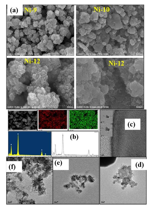
Fig. 7 (a) Field-emission scanning electron microscope (FE-SEM) images of nickel sulfide nanoparticles (NPs) with compositions Ni9, Ni10, and Ni12; (b) energy-dispersive X-ray (EDX), mapping, and line scanning specifically for Ni12; transmission electron microscope (TEM) images showcase (c) Ni2, (d) Ni9, and (e and f) Ni12.36
