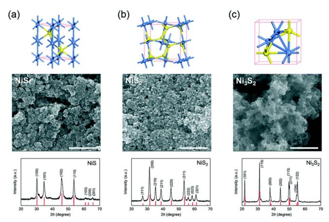
Fig. 4 The unit cell structures, scanning electron microscopy (SEM) images, and X-ray diffraction (XRD) patterns of three nickel sulfides— (a)  $\alpha$ -NiS, (b) NiS<sub>2</sub>, and, (c) Ni<sub>3</sub>S<sub>2</sub>. The red vertical lines in each XRD panel indicate the theoretical pattern.<sup>34</sup>
