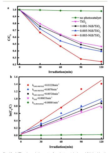
Fig. 12 (a)The degradation rates for photocatalysis and (b) the kinetic curves of methyl orange (MO) degradation for both pure  $TiO_2$  nanosheets arrays (NSAs) and x-NiS/ $TiO_2$  p-n heterostructured NSAs with varying NiS content.<sup>53</sup>
