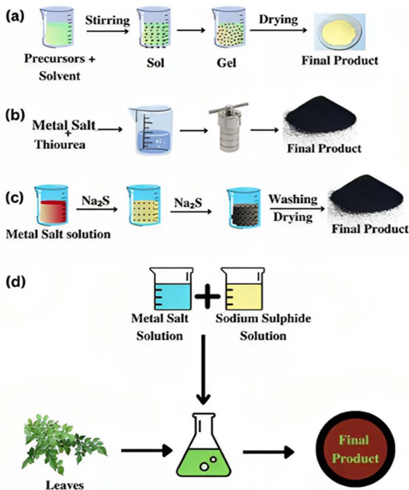
Fig. 3 Graphical depiction of the (a) sol-gel, (b) hydrothermal, (c) precipitation, and (d) green synthesis methods.<sup>10</sup>
