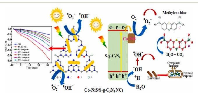
Fig. 14 Pictorial representation of the photocatalytic performance of Co−NiS/q-C<sub>3</sub>N<sub>4</sub> nanocomposite.<sup>63</sup>
