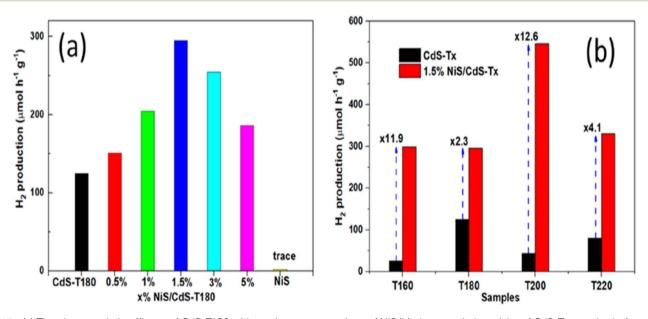
Fig. 13 (a) The photocatalytic efficacy of CdS-T180 with varying concentrations of NiS (b) photocatalytic activity of CdS-T<sub>x</sub> samples before and after the addition of 1.5 wt% NiS for H<sub>2</sub> production.<sup>58</sup>
