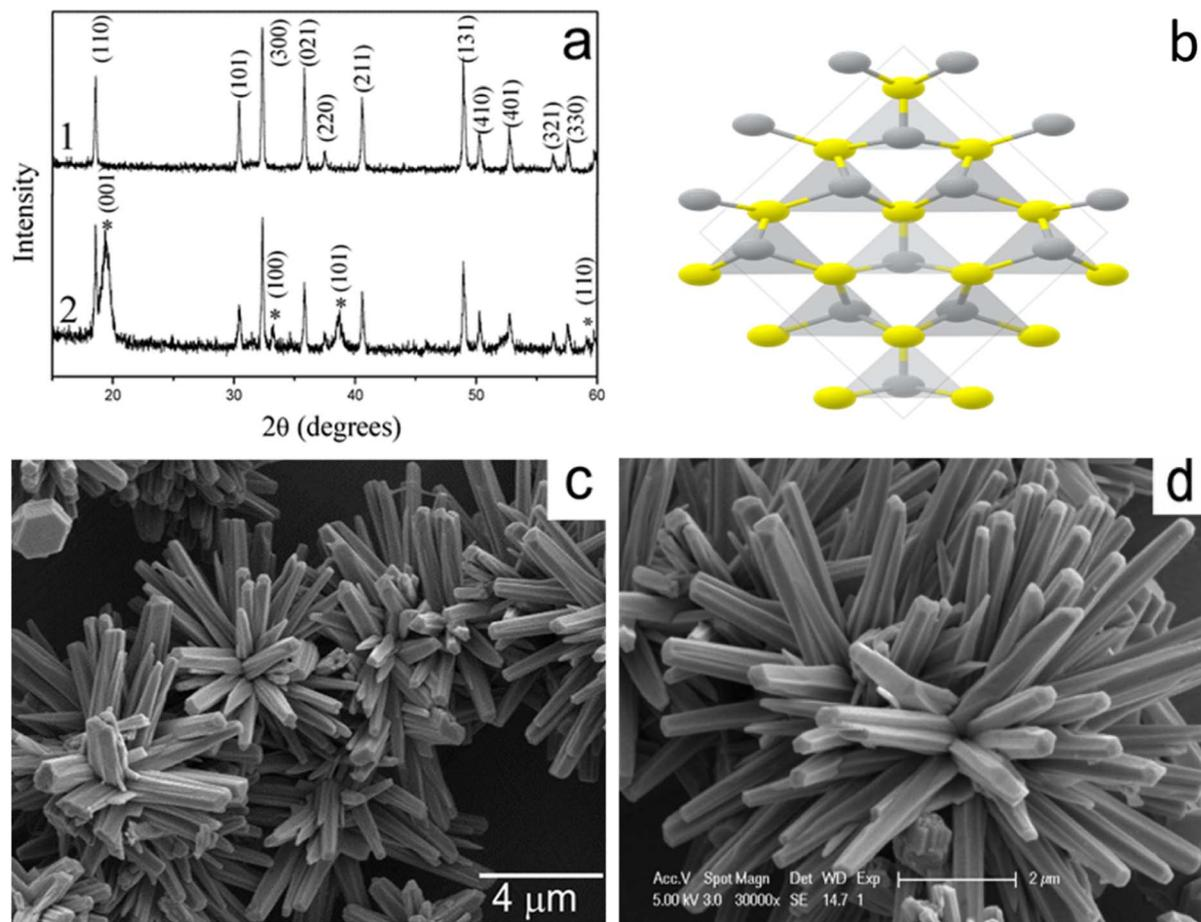
Fig. 5 (a) X-ray diffraction (XRD) patterns, (b) unit cell structures, and (c and d) scanning electron microscopy (SEM) images of  $\beta$ -NiS.<sup>35</sup>
