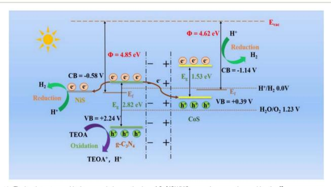
Fig. 16 The band structure and hydrogen evolution mechanism of CoS/CN/NiS composites are under consideration.<sup>67</sup>
