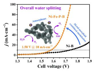
Fig. 10 The overall water-splitting performance of Ni-Fe-P-B@CFP.<sup>47</sup>
