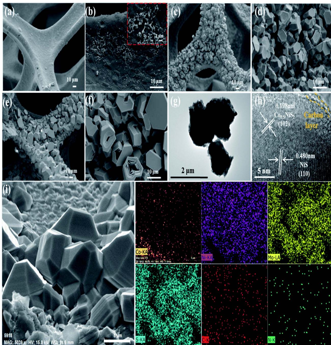
**Fig. 11** (a and b) Mo, Co-NiS/NF-350, (c and d) Mo, Co-NiS/NF-400, and (e and f) Mo, Co-NiS/NF-450 are the synthesized materials' SEM pictures. Furthermore, bulks from Mo, Co-NiS/NF-400 are shown in (g) as TEM pictures, and bulks from the same sources are shown in (h) as HRTEM images. Lastly, (i) shows the Mo, Co-NiS/NF-400 EDS mapping image.<sup>52</sup>
