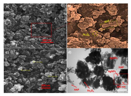
Fig. 2  $Fe_3O_4/HAP/PrNHCS_2H.Ag_{NPs}$ : (a and c) The SEM image of the  $Fe_3O_4@HAp-NH/CS_2@Ag_{NPs}$  and its magnified image (b). (d) TEM image of the Fe<sub>3</sub>O<sub>4</sub>/HAP/PrNHCS<sub>2</sub>H.Ag<sub>NPs</sub>.
