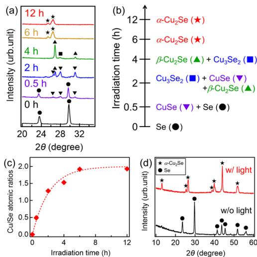
Fig. 4 (a)  $2\theta$ - $\omega$  XRD scans for copper selenide NWs synthesized using UV light irradiation for 0–12 hours. (b) Crystal phases of copper selenide NWs as a function of light irradiation time. (c) Cu/Se atomic ratios obtained by quantitative EDX analysis as a function of light irradiation time. In (c), the dashed curve represents the fitted one to the experimental data with eqn (6). (d)  $2\theta$ - $\omega$  XRD scans for the samples with and without light irradiation for 12 hours.
