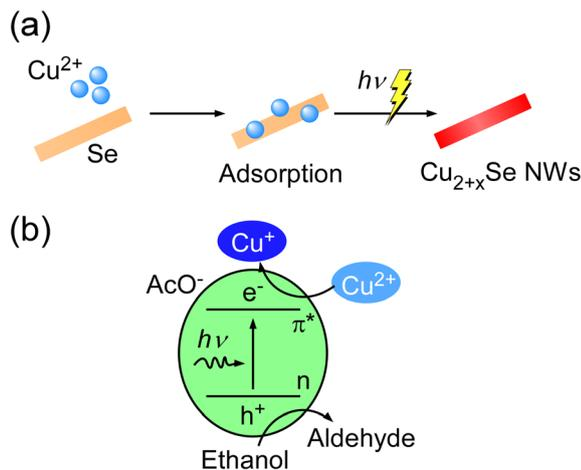
Fig. 5 Schematic illustration of (a) the precise synthesis of  $\text{Cu}_{2+x}\text{Se}$  NWs through photoreduction with  $\text{Cu}^{2+}$  ions adsorbed on Se NWs and (b) the photoreduction mechanism of  $\text{Cu}^{2+}$  ions.
