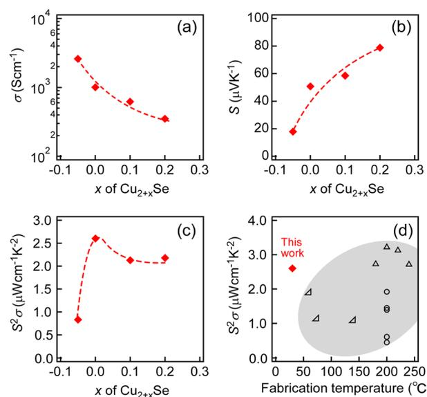
Fig. 3 The composition ratio ( $x$ ) dependencies of (a)  $\sigma$ , (b)  $S$  and (c)  $S^2\sigma$  of Cu<sub>2+x</sub>Se NWs measured at RT. The dashed lines in a–c indicate eye-guides. (d)  $S^2\sigma$  of Cu<sub>2.00</sub>Se NWs (solid symbol) as a function of the fabrication temperature. In (d), the data of polycrystalline films (open symbol)<sup>48–50</sup> were plotted.
