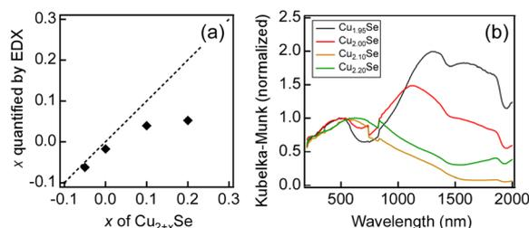
Fig. 2 (a) The composition ratio quantified by EDX ( $x_q$ ) as a function of composition ratio ( $x$ ). The dashed line in (a) indicates the theoretical one when  $x_q$  is the same as  $x$ . (b) DR UV-vis-NIR spectra of Cu<sub>2+x</sub>Se NWs normalized by using the Kubelka–Munk values at around a 500 nm wavelength corresponding to band-edge or interband absorption.
