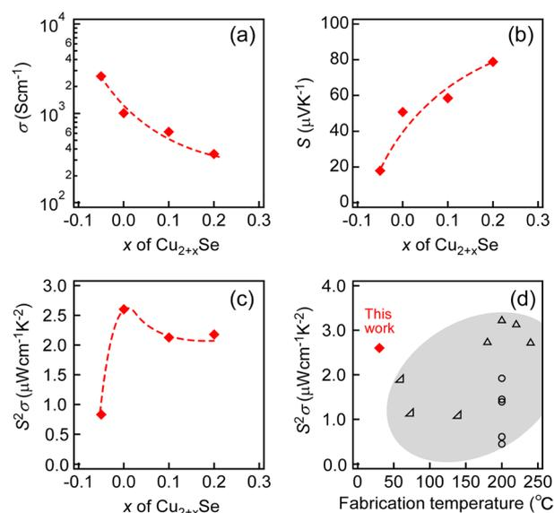
Fig. 3 The composition ratio ( $x$ ) dependencies of (a)  $\sigma$ , (b)  $S$  and (c)  $S^2\sigma$  of Cu<sub>2+x</sub>Se NWs measured at RT. The dashed lines in a–c indicate eye-guides. (d)  $S^2\sigma$  of Cu<sub>2.00</sub>Se NWs (solid symbol) as a function of the fabrication temperature. In (d), the data of polycrystalline films (open symbol)<sup>48–50</sup> were plotted.
