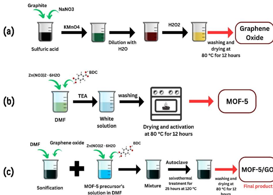
Fig. 1 Scheme for the synthesis of (a) GO, (b) MOF-5, and (c) GO/MOF-5.
