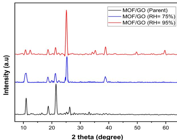
Fig. 7 X-ray diffraction (XRD) patterns for the GO/MOF-5, MOF-5 (75%) and GO/MOF-5 (95%).
