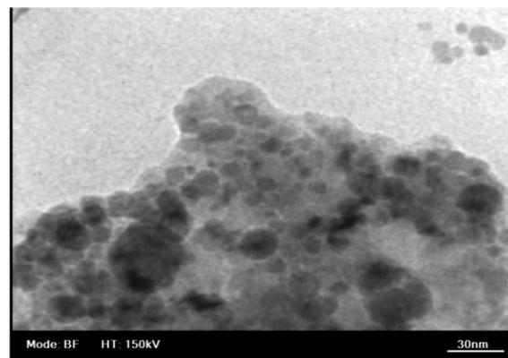
Fig. 4 TEM image of the  $\text{Fe}_3\text{O}_4@SiO_2@Mn$ -complex nanostructure.
