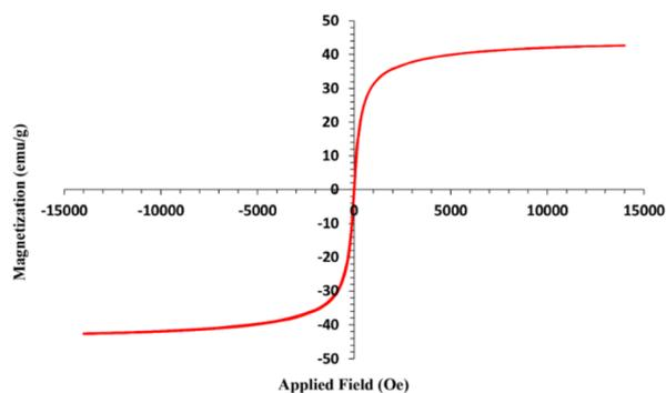
Fig. 6 VSM analysis of  $\text{Fe}_3\text{O}_4@\text{SiO}_2@\text{Mn}$ -complex MNPs.
