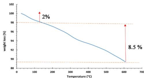
Fig. 5 TGA analysis of  $\text{Fe}_3\text{O}_4@\text{SiO}_2@\text{Mn}$ -complex MNPs.
