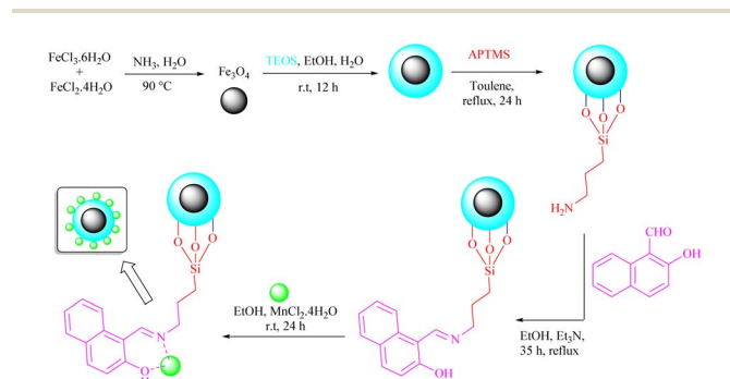
Scheme 3 The pathway for preparation of hybrid MNPs ( \text{Fe}_3\text{O}_4@ \text{SiO}_2@ \text{Mn} -complex).
