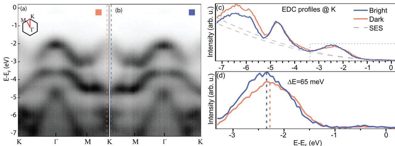
Fig. 6  $\mu\text{ARPES}$  spectra comparing the band structure recorded on (a) dark and (b) bright domains. (c) Difference between the spectral intensity in (a) and (b), highlighting the energy shift between the two. (d) Zoom-in of the region framed in panel (c), highlighting the energy difference between the VBM in the two domains.
