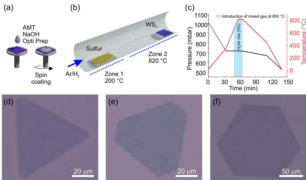
**Fig. 1** Schematic representation of the LiP-CVD growth process; (a) sample preparation with ammonium metatungstate (AMT); (b) graphical representation of the reactor; (c) temperature and pressure ramps during the growth. Bright-field optical images of (d) cut-edge (CE), (e) truncated triangles (TT), (f) hexagonal (HX) shaped CVD grown monolayer  $\text{WS}_2$ .
