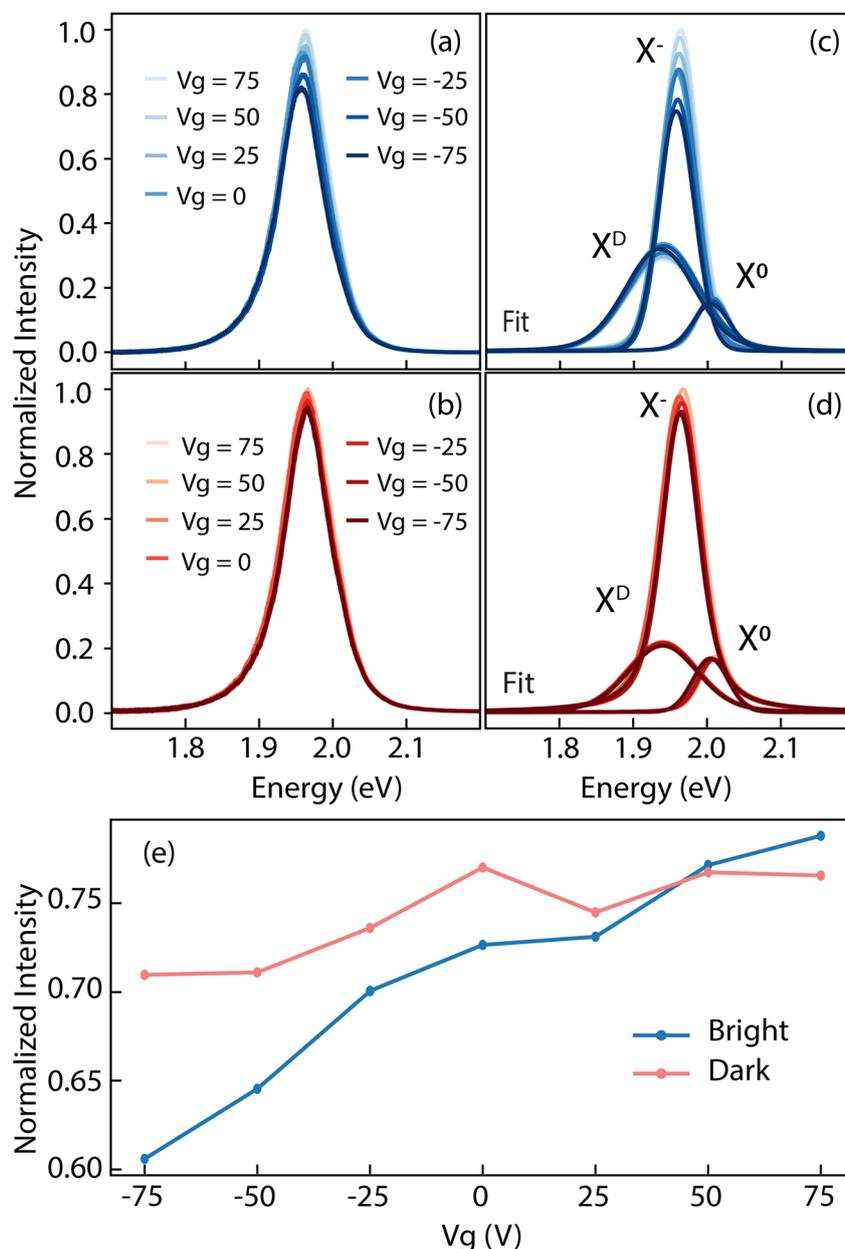
Fig. 7 Gate-dependent PL spectra measured on (a) bright and (b) dark domains. Fitting curve representing neutral ( $X^0$ ), charged ( $X^-$ ) and defect-bound ( $X^D$ ) excitons for bright (c) and dark domains (d). (e) Dispersion of the trion ( $X^-$ ) emission intensity as a function of the gate voltage.
