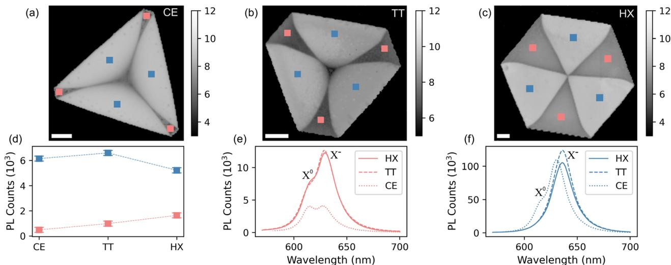
Fig. 3 PL log intensity maps of cut-edged (a), truncated (b), hexagonal (c) monolayer WS<sub>2</sub>. Scalebar 15  $\mu\text{m}$ . (d) Average PL intensity over each domain and shape. (e) Dark domain PL spectra per each shape. (f) Bright domain PL spectra per each shape.
