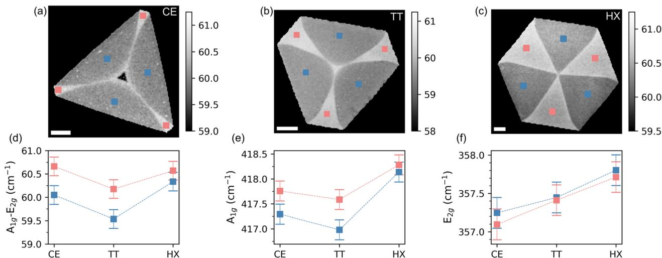
Fig. 2 2D frequency difference maps of (a) cut-edge, (b) truncated, (c) hexagonal shaped monolayer WS<sub>2</sub> measured by Raman spectroscopy. Scalebar 15  $\mu\text{m}$ . (d) Comparisons of frequency difference in the alternating domains of each WS<sub>2</sub>. (e) A<sub>1g</sub> position over each domain and shape (f) E<sub>2g</sub> position over each domain and shape.
