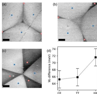
Fig. 5 KPFM maps measured in the central region of each shape. (a) CE, (b) TT and (c) HX flake. Scale bar is 5  $\mu\text{m}$ . (d) Plot indicating the work function difference between bright and dark domains as extracted from KPFM measurements for each shape.
