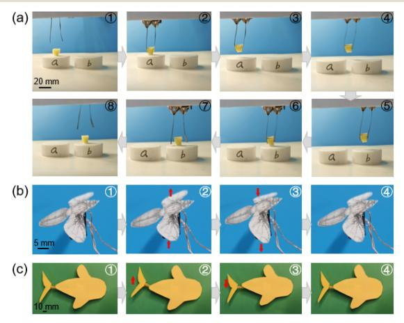
Fig. 5 Bionic applications of the prepared BC-PP-GO/Nafion actuator. (a) Biomimetic gripper utilizing two actuators for manipulating an object. (b) Simulation of a biomimetic fly flapping its wings up and down. (c) A biomimetic fish tail using an actuator.
