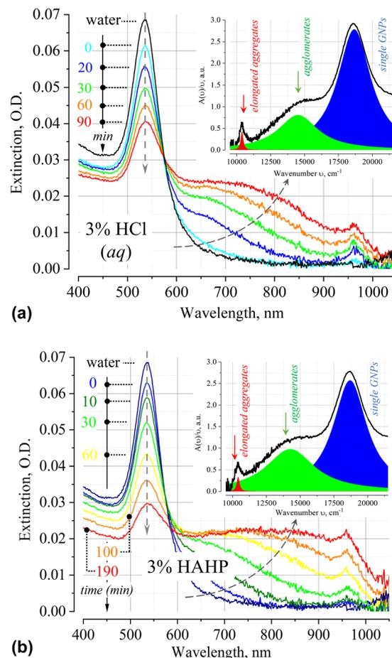
Fig. 2 Time dependence of the extinction spectra for citrate stabilized gold nanoparticles 50 nm in diameter (concentration of single GNPs with  $D_h$  ca. 55 nm  $\sim 3 \times 10^8$  particles per ml) in 3% HCl (aq) (a) and 3% HAHP (b) solutions. The insets show a typical deconvolution of the spectra into individual components with a Lorentzian profile for time  $t = 30$  min after the addition of nanoparticles to the working solutions.
