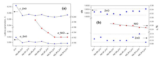
Fig. 3 Influence of dopants on (a) the lattice parameters of phases and (b) the c/a ratio for ZnO and lattice disturbance for the structures of ZnO and NiO
