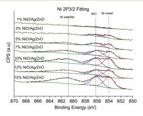
Fig. 6 Ni  $2p_{3/2}$  spectrum obtained from the XPS spectra of Ag-doped and Ni co-doped ZnO NPs.
