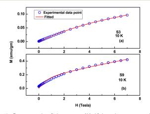
Fig. 17 Representative fitting curves (M-H) based on a core-shell model. (a) S3 (ZnO/Ag/1% NiO) and (b) S9 (ZnO/Ag/15% NiO).
