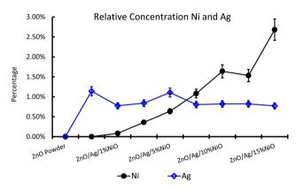
Fig. 8 Relative concentration of Ag and Ni in Ag-doped and Ni codoped ZnO NPs.
