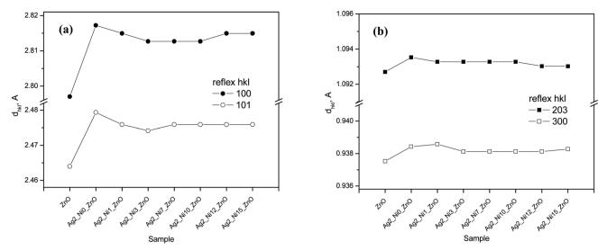
Fig. 2 Influence of dopants on principal inter-plane distances  $d_{nkl}$  for the structure of (a) Ag-doped and (b) Ni co-doped ZnO NPs.
