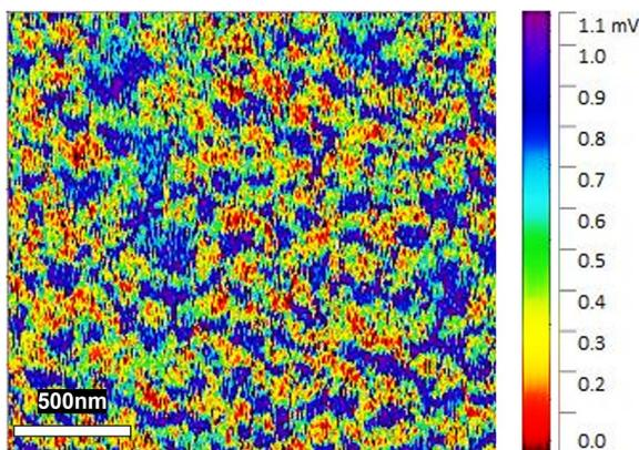
Fig. 4 KFPM image of Pt#CeO<sub>2</sub>/Si, where the contrast from cold to warm colors visualizes the surface potential of the sample relative to the Pt probe surface.
