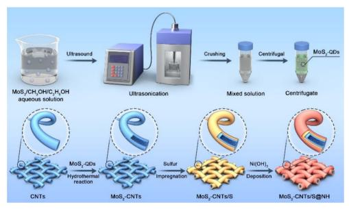
Fig. 1 Schematic of the synthesis process of MoS<sub>2</sub> QDs-CNTs/S@NH composites.
