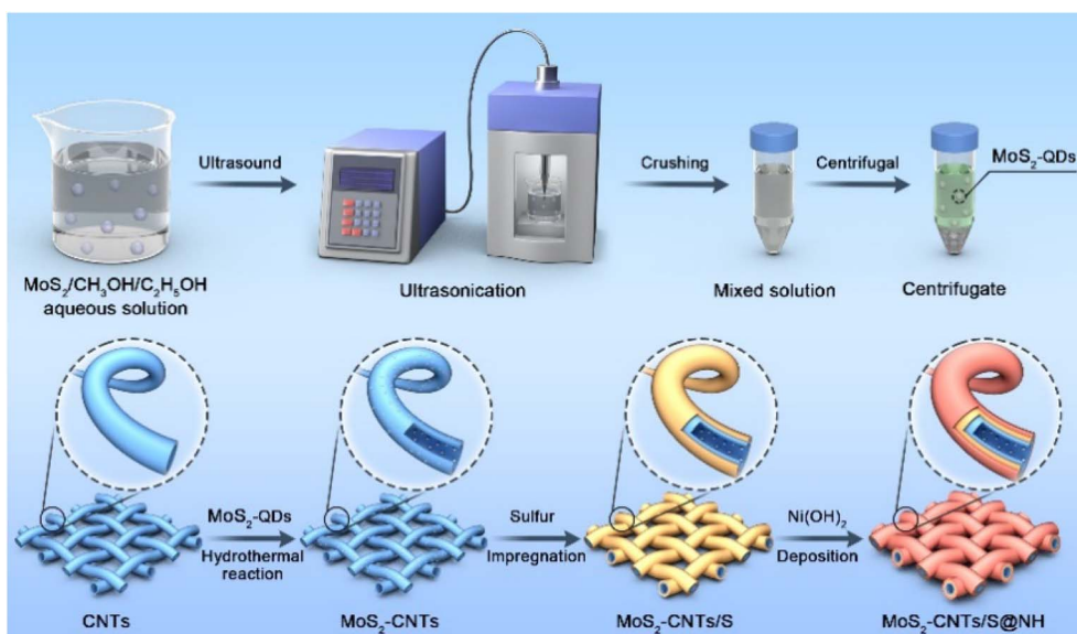
Fig. 1 Schematic of the synthesis process of MoS 2 QDs-CNTs/S@NH composites.
