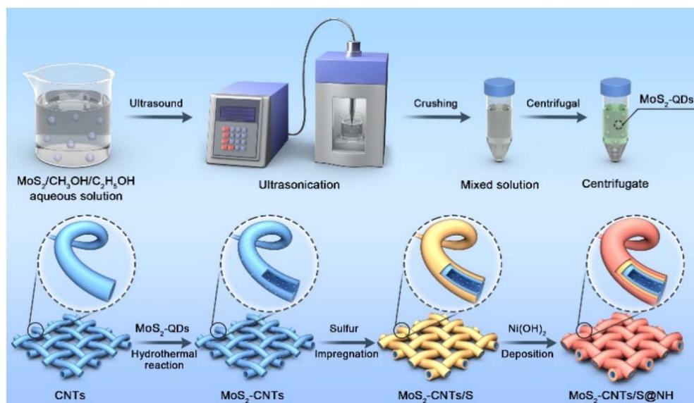
Fig. 1 Schematic of the synthesis process of MoS<sub>2</sub> QDs-CNTs/S@NH composites.
