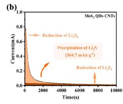
Fig. 6 Potentiostatic discharge curves of CNTs and MoS<sub>2</sub> QDs-CNTs.
