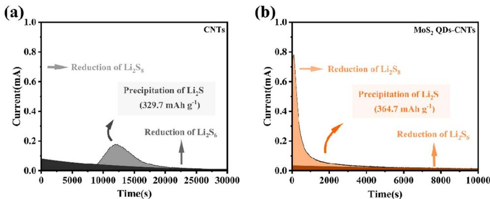
Fig. 6 Potentiostatic discharge curves of CNTs and MoS<sub>2</sub> QDs-CNTs.
