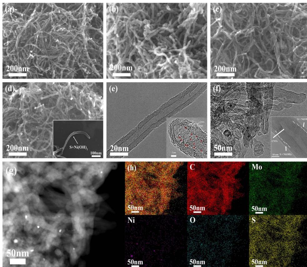
Fig. 2 SEM images of (a) CNTs, (b) MoS<sub>2</sub> QDs-CNTs, (c) MoS<sub>2</sub> QDs-CNTs/S, and (d) MoS<sub>2</sub> QDs-CNTs/S@NH. (e) HRTEM image of MoS<sub>2</sub> QDs-CNTs. (f and g) High-magnification TEM image of MoS<sub>2</sub> QDs-CNTs/S@NH and the EDS mapping.
