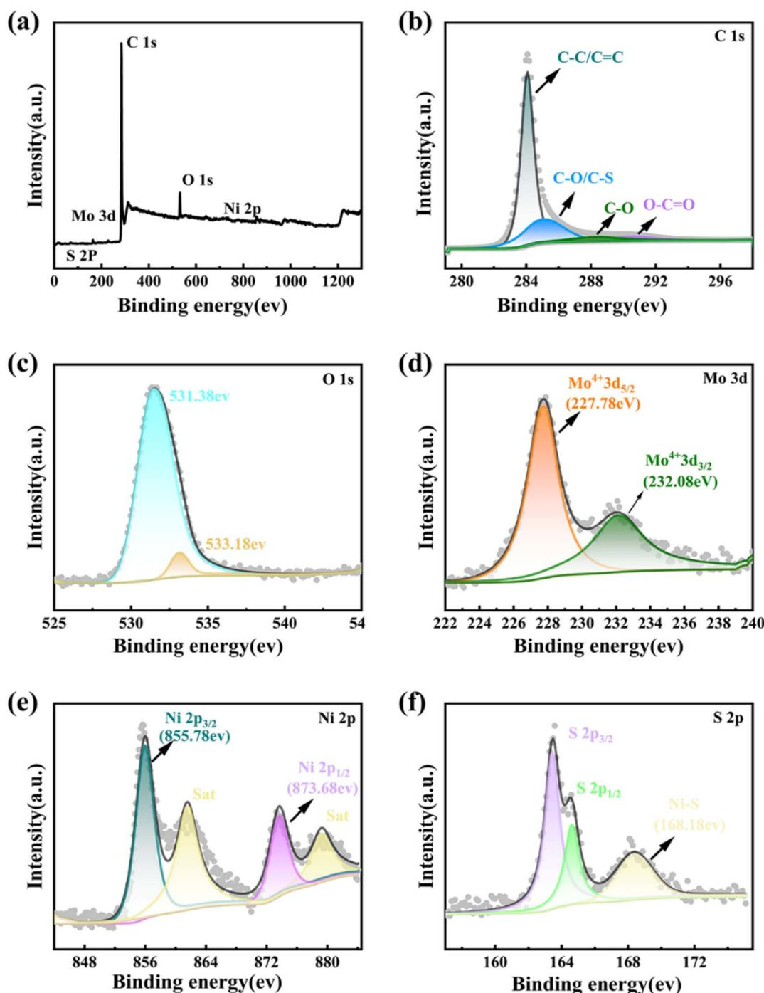
Fig. 4 XPS spectra of the MoS<sub>2</sub> QDs-CNTs/S@NH sample: (a) overall XPS spectrum, (b) C 1s, (c) O 1s, (d) Mo 3d, (e) Ni 2p, and (f) S 2p XPS spectra.
