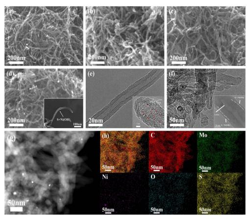
Fig. 2 SEM images of (a) CNTs, (b) MoS<sub>2</sub> QDs-CNTs, (c) MoS<sub>2</sub> QDs-CNTs/S, and (d) MoS<sub>2</sub> QDs-CNTs/S@NH. (e) HRTEM image of MoS<sub>2</sub> QDs-CNTs/S, and (d) MoS<sub>2</sub> QDs-CNTs/S@NH. CNTs. (f and g) High-magnification TEM image of MoS<sub>2</sub> QDs-CNTs/S@NH and the EDS mapping.
