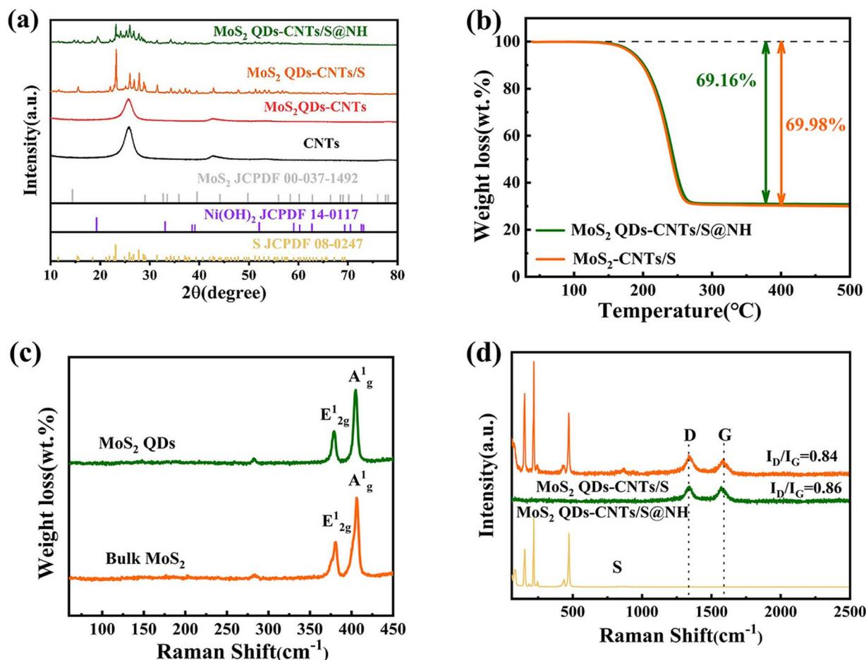
Fig. 3 (a) XRD patterns of S, CNTs, MoS<sub>2</sub> QDs-CNTs, Ni(OH)<sub>2</sub>, MoS<sub>2</sub> QDs-CNTs/S and MoS<sub>2</sub> QDs-CNTs/S@NH composite materials; (b) TG curves of MoS<sub>2</sub> QDs-CNTs/S and MoS<sub>2</sub> QDs-CNTs/S@NH; (c) Raman spectra of MoS<sub>2</sub> QDs and bulk MoS<sub>2</sub>. (d) Raman spectra of MoS<sub>2</sub> QDs-CNTs/S and MoS<sub>2</sub> QDs-CNTs/S@NH.
