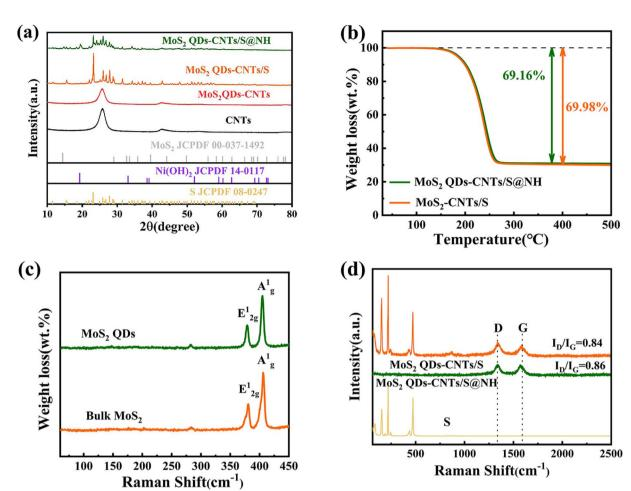
Fig. 3 (a) XRD patterns of S, CNTs, MoS<sub>2</sub> QDs-CNTs, Ni(OH)<sub>2</sub>, MoS<sub>2</sub> QDs-CNTs/S and MoS<sub>2</sub> QDs-CNTs/S@NH composite materials; (b) TG curves of MoS<sub>2</sub> QDs-CNTs/S and MoS<sub>2</sub> QDs-CNTs/S@NH; (c) Raman spectra of MoS<sub>2</sub> QDs and bulk MoS<sub>2</sub>. (d) Raman spectra of MoS<sub>2</sub> QDs-CNTs/S@NH.
