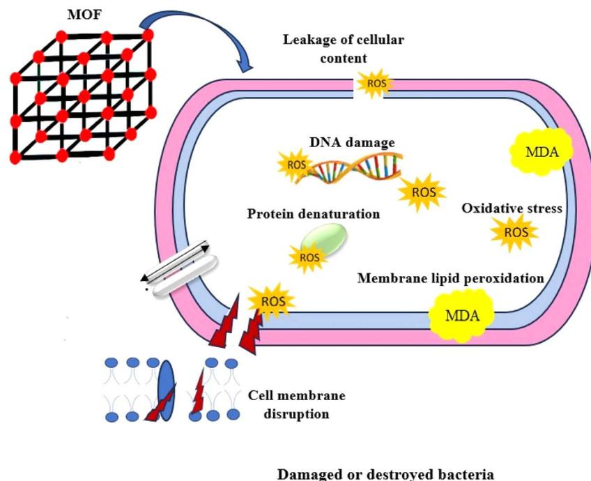
Fig. 3 Schematic mechanism of antibacterial activity of Ag-MOF.
