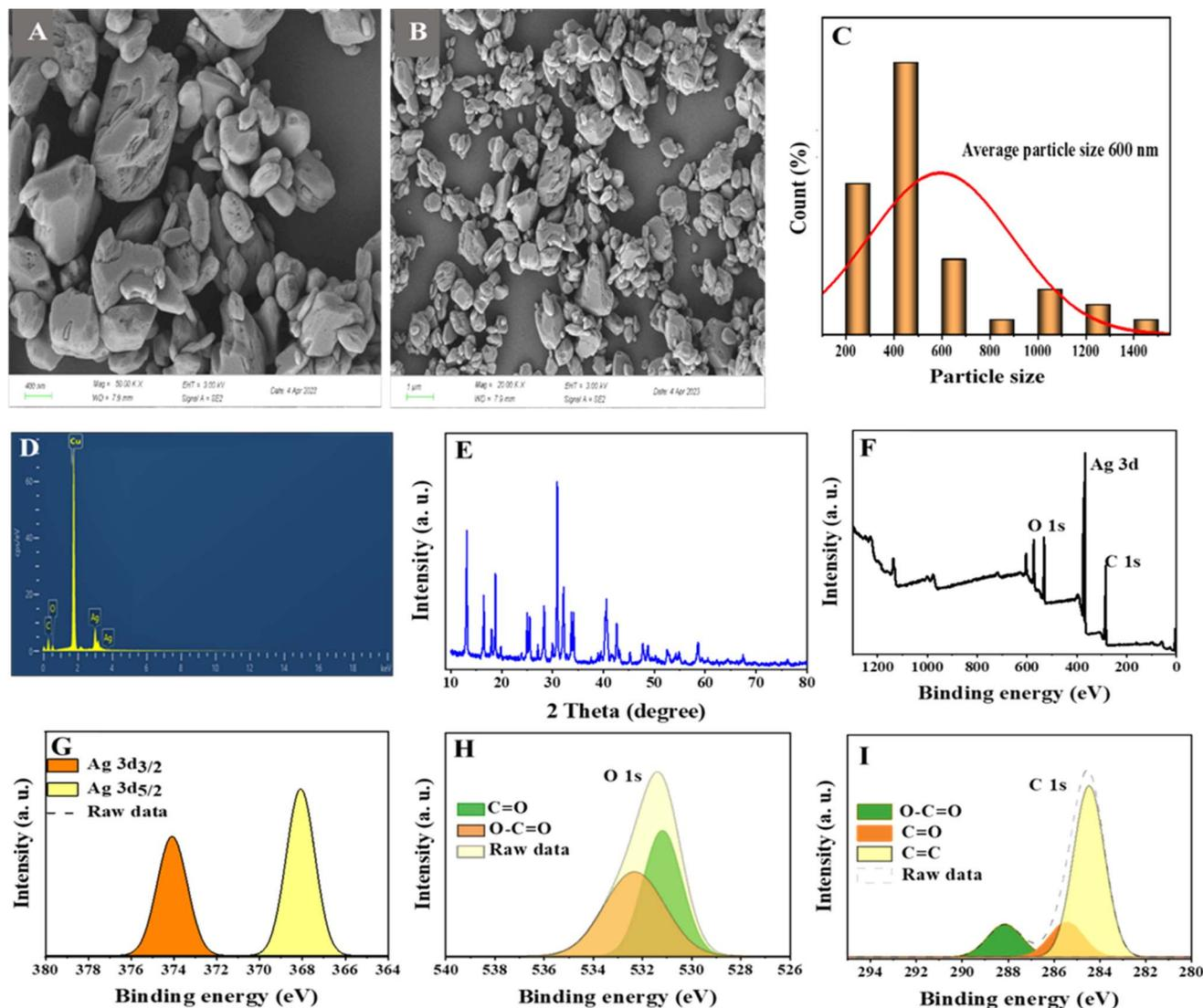
Fig. 1 (A and B) FE-SEM images of the Ag-MOF. (C) Histogram of particle size diameter of Ag-MOF. (D) EDX image of the synthesized Ag-MOF. (E) XRD spectrum of the Ag-MOF. (F) Survey XPS spectrum of the Ag-MOF. Deconvoluted spectra of the elements in the synthesized Ag-MOF. (G) Ag 3d. (H) O 1s. (I) C 1s.
