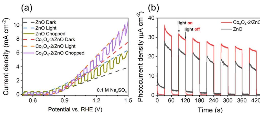
Fig. 6 Light-chopped LSV curves (a) and photocurrent density response (b) of ZnO and  $\text{Co}_3\text{O}_4\text{-2/ZnO}$  samples.
