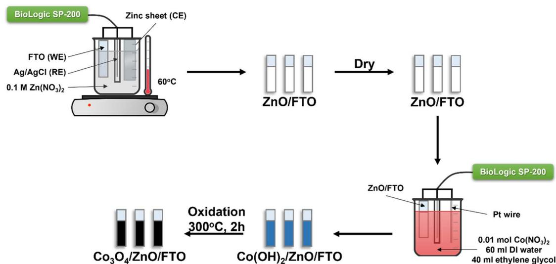
Scheme 1 Schematic illustration of the preparation of  $\text{Co}_3\text{O}_4/\text{ZnO}/\text{FTO}$ .
