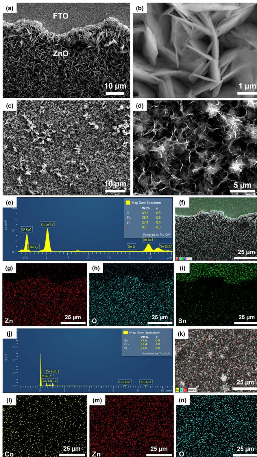
Fig. 2 SEM images of the ZnO/FTO sample at magnifications (a) 2000 $\times$ , (b) 20 000 $\times$ ; SEM images of the Co<sub>3</sub>O<sub>4</sub>/ZnO/FTO sample at magnifications (c) 2000 $\times$ , (d) 5000 $\times$ ; EDX-mapping of ZnO/FTO (e–i) and Co<sub>3</sub>O<sub>4</sub>/ZnO/FTO (j–n).
