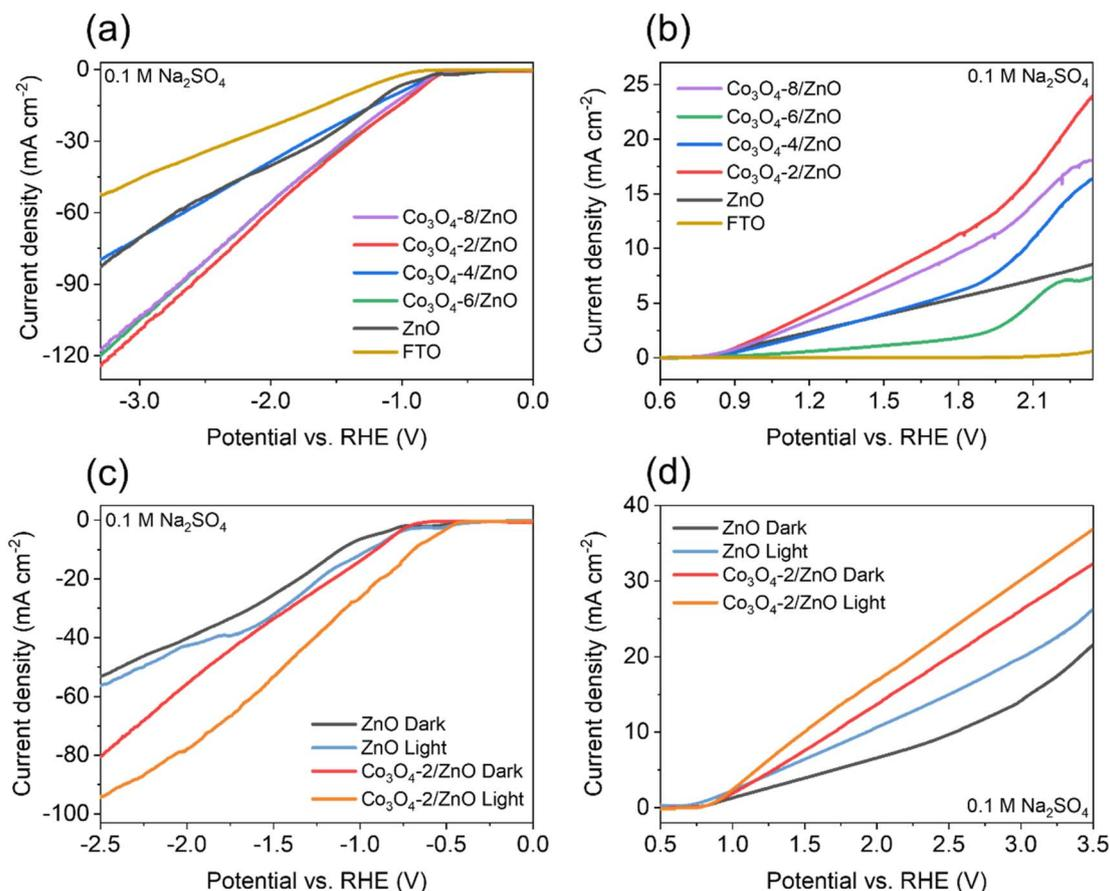
Fig. 5 HER (a) and OER (b) curves of FTO, ZnO and  $\text{Co}_3\text{O}_4/\text{ZnO}$  samples; HER (c) and OER (d) curves of ZnO and  $\text{Co}_3\text{O}_4\text{-2}/\text{ZnO}$  samples under the illuminated and non-illuminated conditions.
