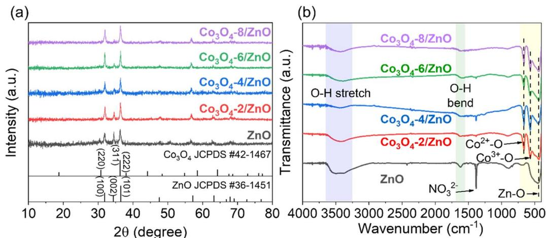
Fig. 1 XRD patterns (a) and FTIR spectra (b) of ZnO/FTO and  $\text{Co}_3\text{O}_4/\text{ZnO}/\text{FTO}$  samples.
