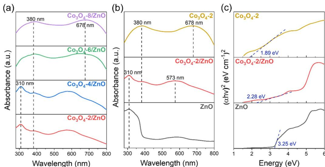
Fig. 3 DRS spectra of the synthesized  $\text{Co}_3\text{O}_4/\text{ZnO}$  samples with different deposition times (a); DRS spectra (b) and Tauc plots (c) of synthesized ZnO,  $\text{Co}_3\text{O}_4-2$ ,  $\text{Co}_3\text{O}_4-2/\text{ZnO}$  samples.
