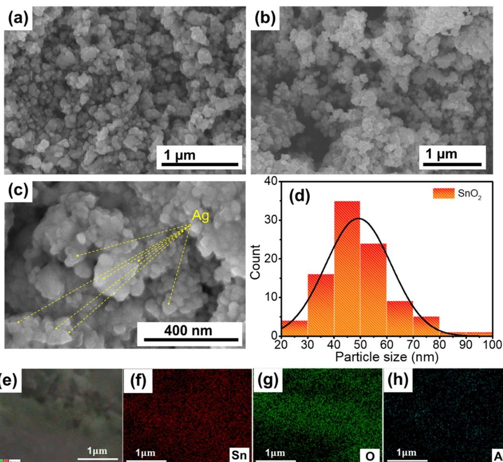
Fig. 2 SEM images of (a) SnO<sub>2</sub> and (b and c) Ag TNPs/SnO<sub>2</sub>; (c) particle size distribution histogram of SnO<sub>2</sub> in the Ag TNPs/SnO<sub>2</sub> sample; (e-h) SEM-EDS elemental mapping of Ag TNPs/SnO<sub>2</sub>.
