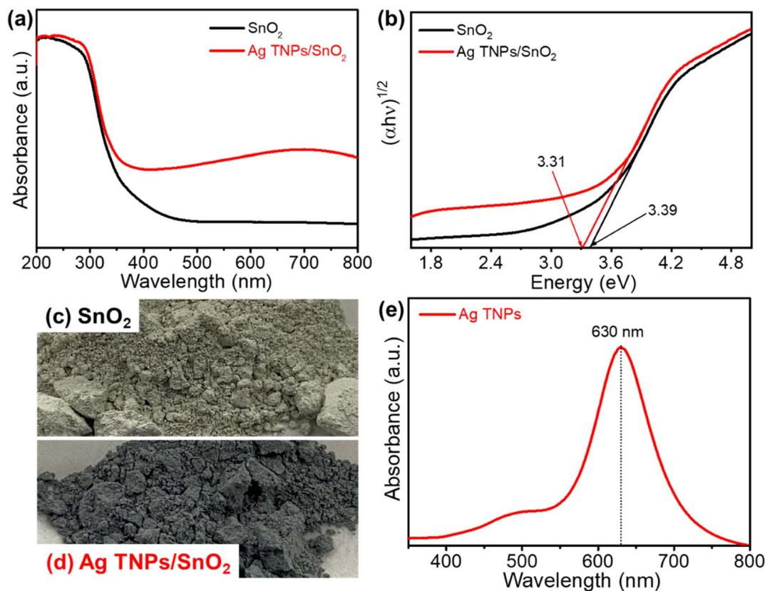
Fig. 3 (a) UV-Vis DRS and (b) Tauc plots of SnO<sub>2</sub> and Ag TNPs/SnO<sub>2</sub>; (c and d) optical images of as-prepared SnO<sub>2</sub> and Ag TNPs/SnO<sub>2</sub>; (e) UV-Vis absorption spectrum of Ag TNPs.
