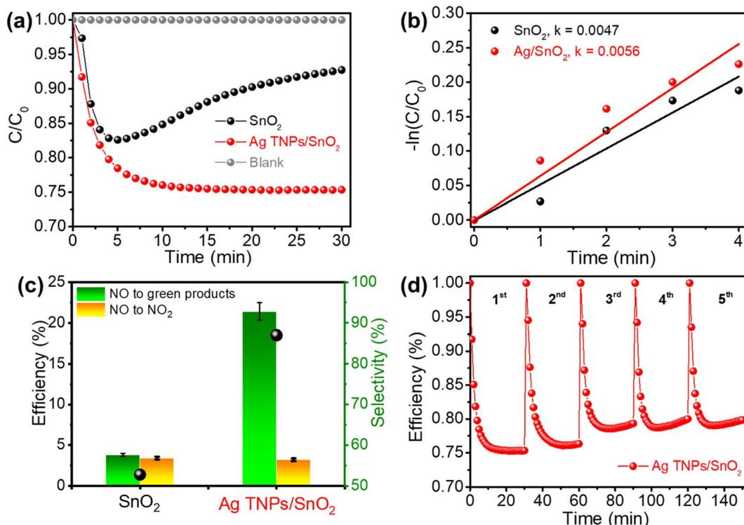
Fig. 5 (a and b) Photocatalytic NO removal ability and kinetic rates, (c) NO to NO<sub>2</sub> and NO<sub>3</sub><sup>-</sup> conversion efficiencies over SnO<sub>2</sub> and Ag TNPs/SnO<sub>2</sub>; (d) stability test of photocatalytic NO removal over Ag TNPs/SnO<sub>2</sub>.
