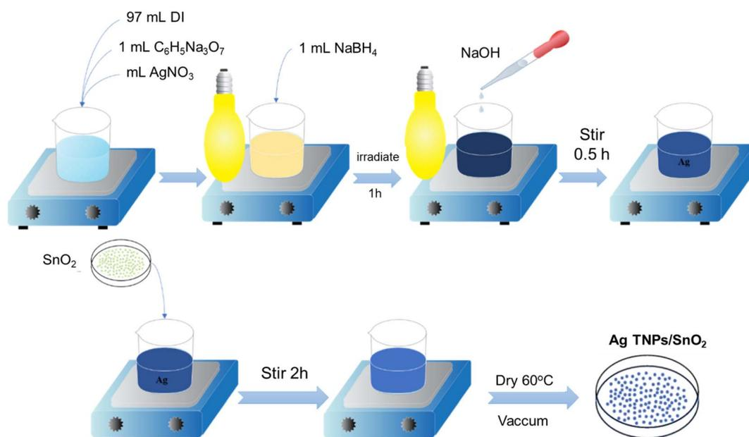
Scheme 1 Synthesis process of Ag TNPs/SnO<sub>2</sub>.
