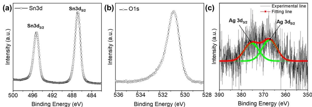
Fig. 4 High-resolution XPS of Ag TNPs/SnO<sub>2</sub>: (a) Sn 3d, (b) O 1s, and (c) Ag 3d.
