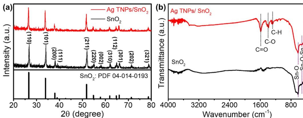
Fig. 1 (a) XRD patterns and (b) FTIR spectra of SnO<sub>2</sub> and Ag TNPs/SnO<sub>2</sub>.
