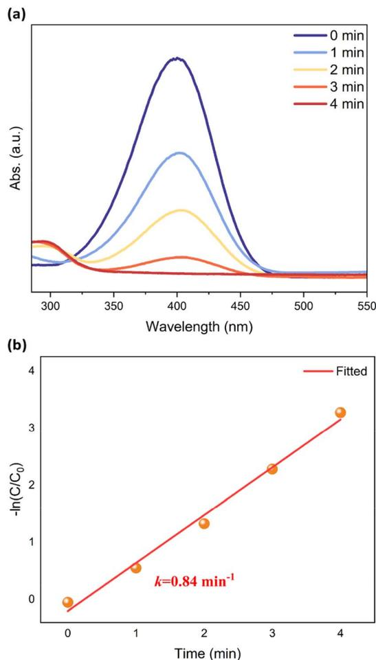
Fig. 5 (a) UV-vis spectra showing the gradual reduction of 4-NP in the presence of **Cu<sub>6</sub>-3** and (b) plot of  $-\ln(C/C_0)$  versus time.
