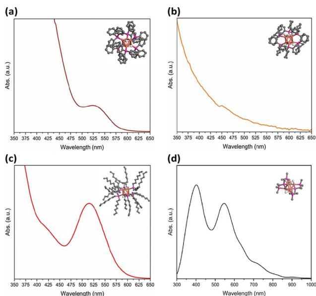
Fig. 2 The experimental UV-vis absorption spectra of (a) **Cu<sub>6</sub>-1**, (b) **Cu<sub>6</sub>-2**, (c) **Cu<sub>6</sub>-3** and (d) TDDFT simulated absorption spectrum of  $[\text{CuH}]_6$  (the Gaussian width was set to 60 nm). Insets show their structures. Colour legend: orange, Cu; pink, P; grey, C; white, H. Hydrogen atoms on ligands are omitted for clarity.
