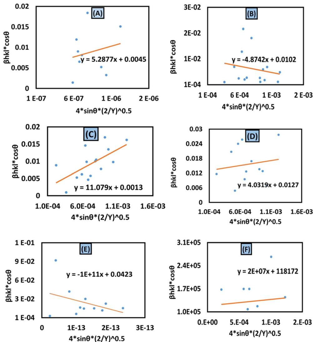
Fig. 8 Uniform deformation energy density model for calculating crystallite size for (A) 50% ethanoL\_HAp, (B) 100% ethanoL\_HAp, (C) 50% IPA\_HAp, (D) urea\_HAp, (E) palmitic acid\_HAp and (F) naphthalene\_HAp.
