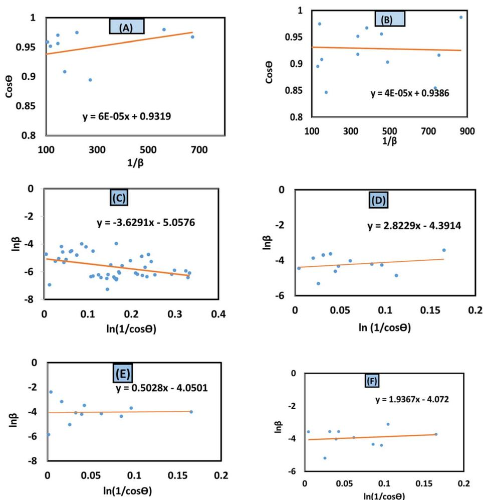
Fig. 4 Linear straight-line model of Scherrer's equation for crystallite size estimation for (A) 50% ethanol\_HAp, (B) 100% ethanol\_HAp, (C) 50% IPA\_HAp, (D) urea\_HAp, (E) palmitic acid and (F) naphthalene\_HAp.
