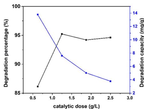
Fig. 14 Effect of various dosages (0.625, 1.25, 1.875, and 2.5 g L<sup>-1</sup>) of the photocatalyst with fixed 10 ppm of 40 mL Congo red dye, 0.05 g of catalyst, and 90 min time on 100% ethanoL\_HAp.
