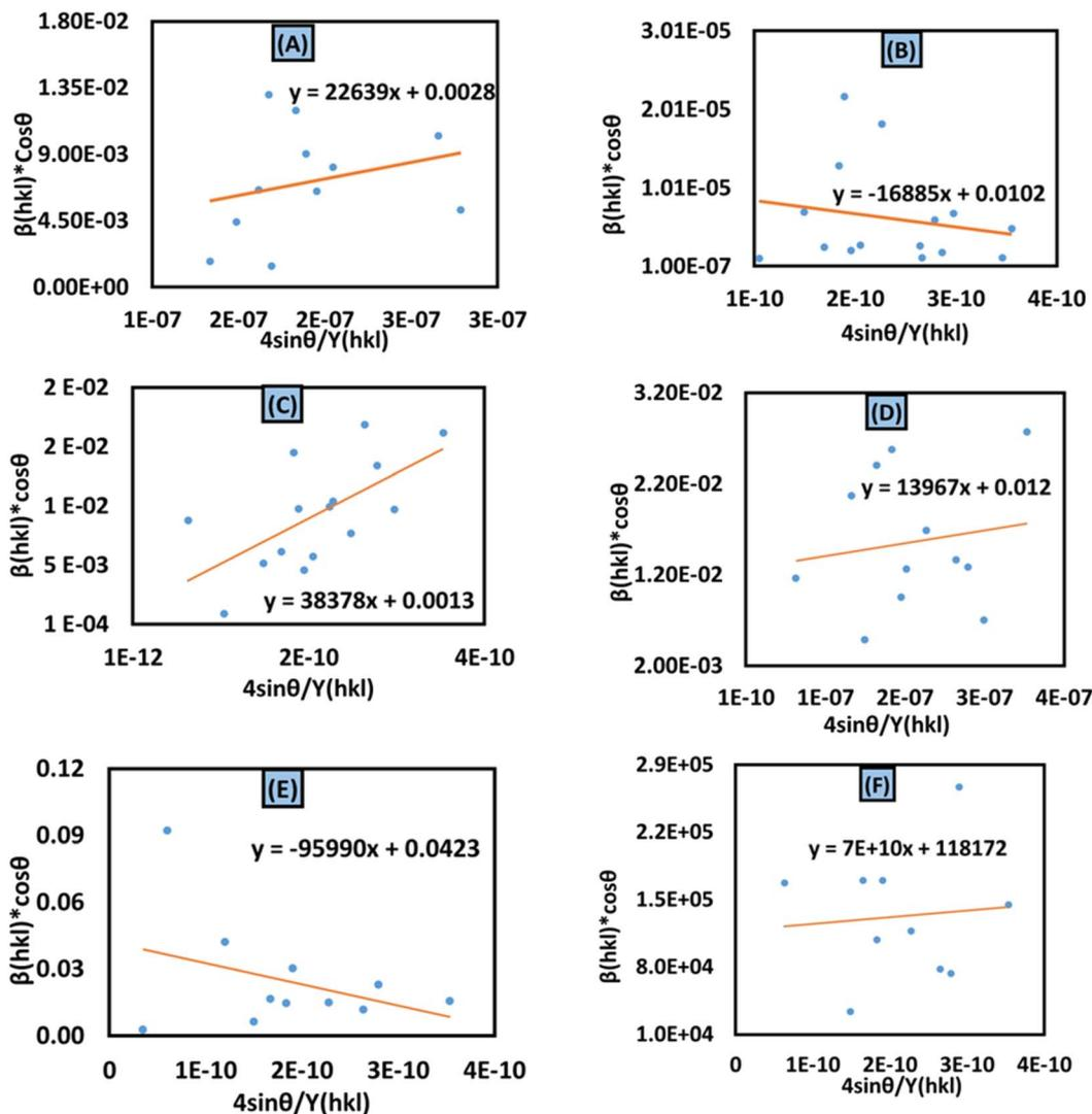
Fig. 7 Uniform stress deformation model for calculating crystallite size for (A) 50% ethanoL\_HAp, (B) 100% ethanoL\_HAp, (C) 50% IPA\_HAp, (D) urea\_HAp, (E) palmitic acid\_HAp and (F) naphthalene\_HAp.
