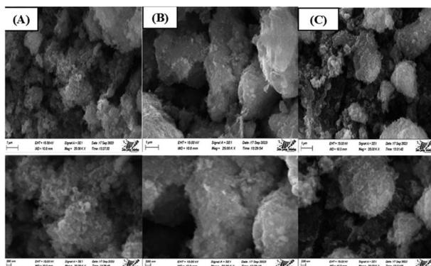
Fig. 12 Scanning electron micrograph of Synthesized HAP using different modifiers, (A) urea, (B) palmitic acid, and (C) naphthalene.
