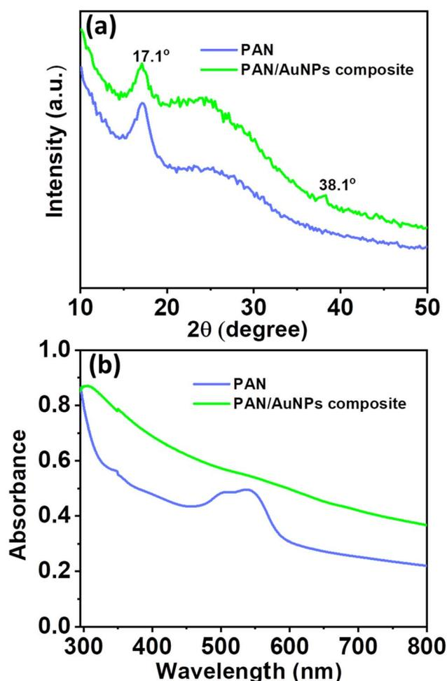
Fig. 3 (a) XRD and (b) UV visible spectra of PAN and PAN/AuNPs composite film.
