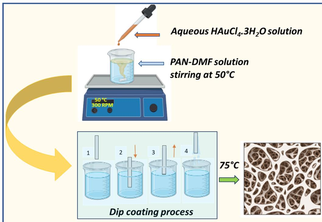
Fig. 1 Schematic representation of SERS substrate preparation.
