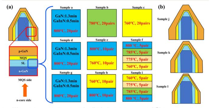
Fig. 1 (a) Schematic diagrams of the NW samples with GalnN/GaN SLs. The detailed structures on the  $(10\overline{10})$ -plane are illustrated from the n-core side to the p-GaN shell. The detailed growth conditions of SLs in three different batches of NW samples are shown in the left, while the bottom represents the n-core side and the upper side represents the MQS side. (b) Schematic diagrams of the NW samples j, k, and l with different p-GaN growth times.
