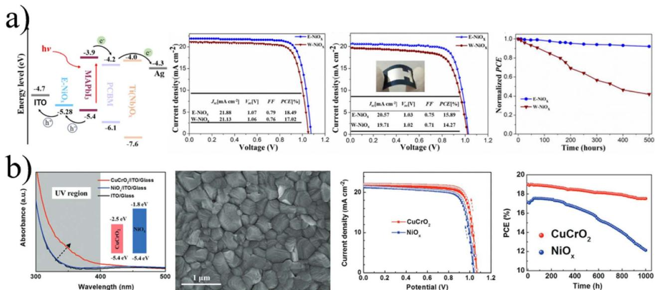
Fig. 3 (a) Energy level diagram of the materials used in the device,  $J$ - $V$  curves of rigid and flexible PSCs, normalized PCE. (b) UV-vis spectra of the CuCrO<sub>2</sub> and NiO<sub>x</sub> layer with optimum thickness with energy level in the inset. Adapted with permission.<sup>87,94</sup> Copyright 2018, Wiley-VCH.
