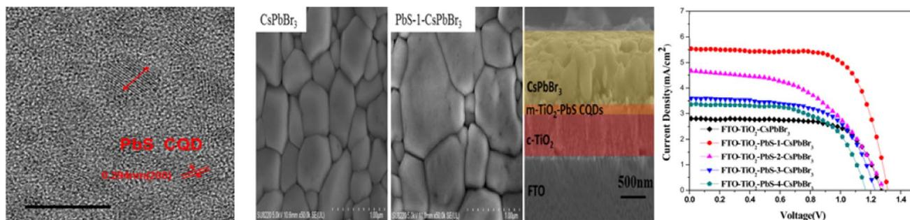
Fig. 12 Top-view and cross-section images of CsPbBr<sub>3</sub> film decorated with PbS NCs, and J–V curves of all-inorganic PSCs based on different TiO<sub>2</sub>/PbS photoanodes. Adapted with permission.<sup>243</sup> Copyright 2019, American Chemical Society.
