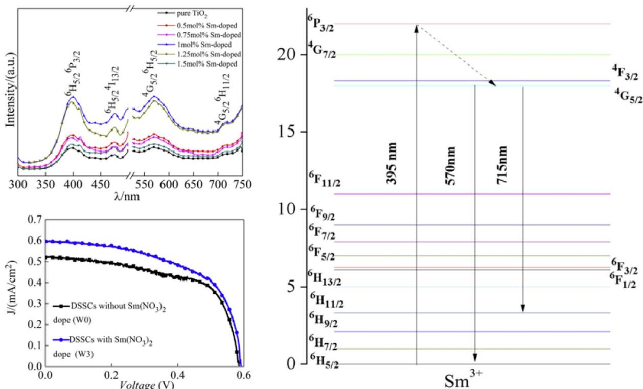
Fig. 15 Excitation spectrum ( $\lambda_{em} = 567$  nm) and emission spectrum ( $\lambda_{ex} = 395$  nm) of  $\text{TiO}_2:\text{Sm}^{3+}$  NCs with different  $\text{Sm}^{3+}$  doping concentrations, and schematic energy-level diagrams to show the details of down-conversion mechanisms *via* excitation using 395 nm radiation for  $\text{TiO}_2:\text{Sm}^{3+}$  NCs. Adapted with permission.<sup>244</sup> Copyright 2016, Elsevier.
