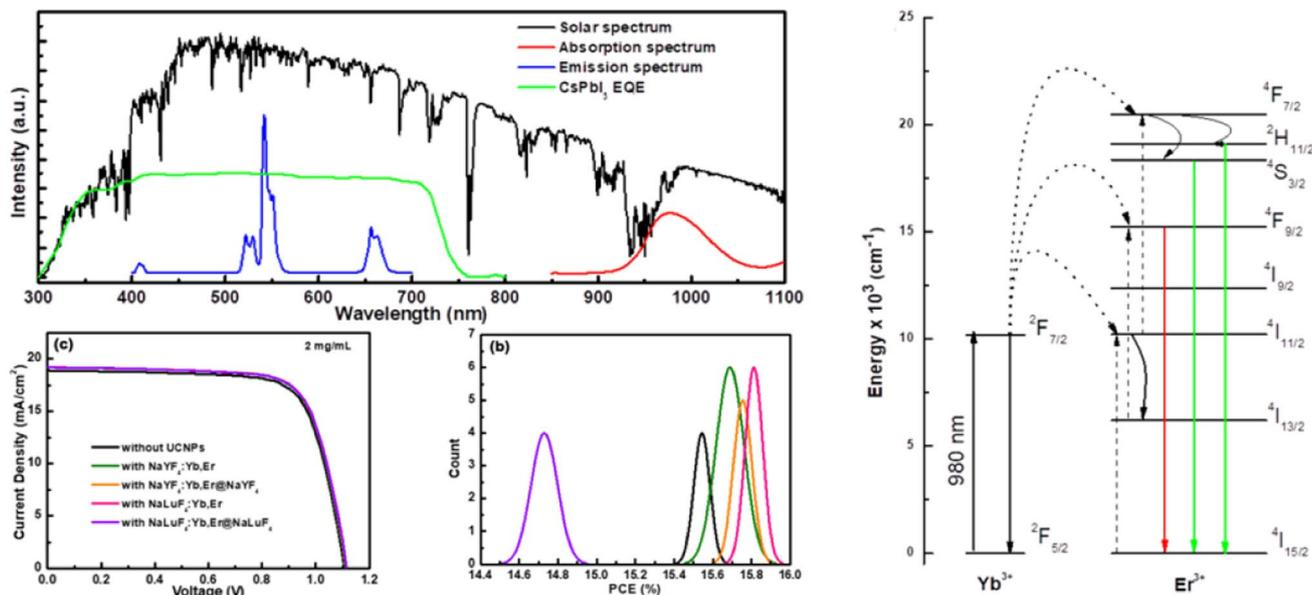
Fig. 14 Solar spectrum, absorption and emission spectrum of up-conversion nanocrystals and EQE curve of  $\gamma$ -CsPbI<sub>3</sub> PSC,  $J$ - $V$  curves of PSCs based on different nanocrystals, and statistical PCE distribution histograms of 30 devices, schematic energy diagram for Yb<sup>3+</sup> and Er<sup>3+</sup>. Adapted with permission.<sup>237</sup> Copyright 2019, American Chemical Society.
