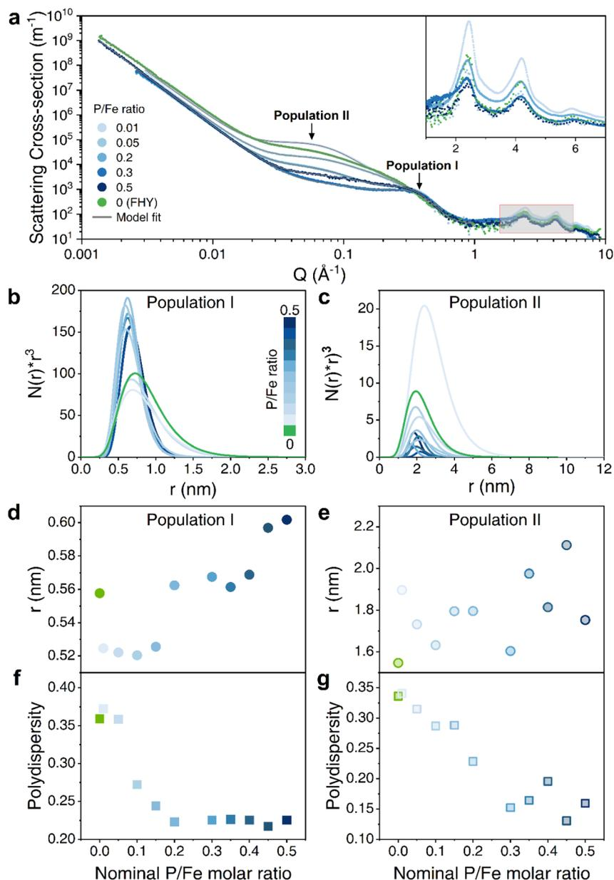
**Fig. 3** (a) SAXS curves for FHY and coprecipitates synthesized at different P/Fe ratios (both axes are log 10 scale) and the inset is the enlarged grey WAXS region (linear scale). Size distribution, variations in the average radius and polydispersity for the primary beads (population I) (b, d and f) and the nanoparticles (c, e and g).
