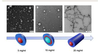
Fig. 1 TEM images and schematic representation of self-assembled PHPMA-g-PLA at different  $C_{\rm final}$ : (A) Ms at 0.5 wt%, (B) Vs at 1.0 wt% and (C) Ws at 2.0 wt%.
