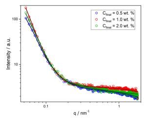
Fig. 2 SAXS curves for PHPMA-q-PLA NPs formed in microfluidic channels at different  $C_{\text{final}}$ : 0.5 wt% (Ms, blue circles), 1.0 wt% (Vs, red circles), and 2.0 wt% (Ws, green circles)
