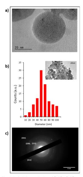
Fig. 1 Morphological characterization of Si-NPs. Si-NPs were characterized by HR-TEM analysis (a). Si-NP size distribution is displayed in histogram (b) where the bars show the percentage of Si-NPs for the different sizes indicated on the x-axis. (c) Electron diffraction pattern of Si-NPs.
