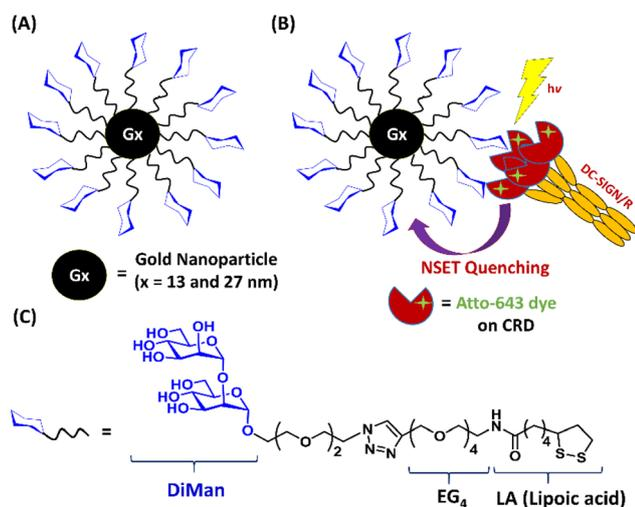
**Fig. 1** (A) Schematic structure of Gx-DiMan; (B) our approach to probe DC-SIGN/R binding with Gx-DiMan *via* GNP fluorescence quenching: upon binding, the excited energies of fluorophore labels on DC-SIGN/R are efficiently transferred to the proximal Gx-DiMan *via* the NSET mechanism, leading to a greatly reduced fluorescence signal. (C) Chemical structure of the LA-EG<sub>4</sub>-DiMan ligand.
