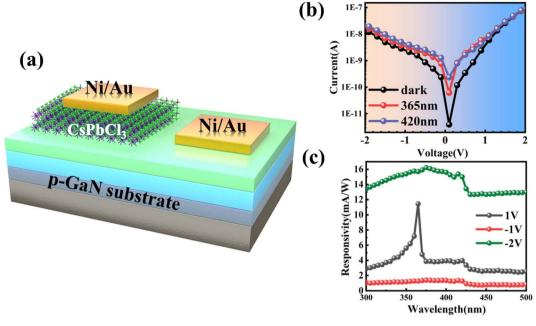
Fig. 3 (a) Schematic diagram of the CsPbCl<sub>3</sub>/GaN heterojunction photodetector; (b) I-V characteristic curves of the device under dark conditions, 365 nm illumination and 420 nm illumination; (c) photoresponse of devices in the visible – ultraviolet range at bias voltages of 1V, –1V and -2 V.
