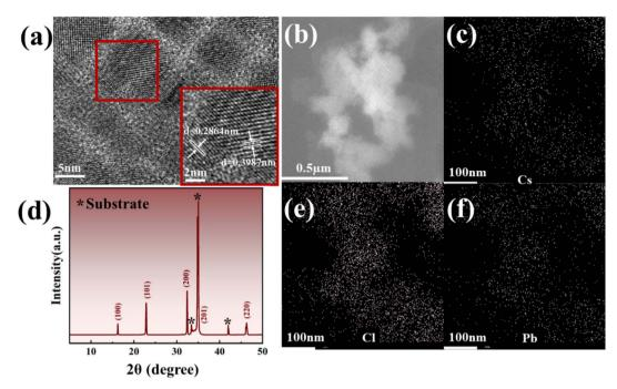
Fig. 2 (a) TEM analysis image of CsPbCl<sub>3</sub>; (b) EDS scanning area; (c), (e) and (f) EDS mapping images of each element of CsPbCl<sub>3</sub>; (d)  $\omega$ -2 $\theta$  XRD scan of CsPbCl<sub>3</sub>.
