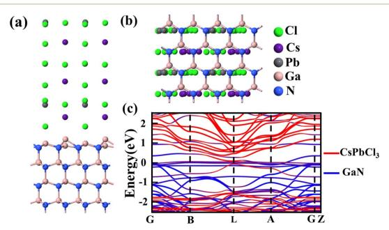
Fig. 4 (a) Side view; (b) top view; (c) projected energy band diagram of the CsPbCl<sub>3</sub>/GaN heterojunction.
