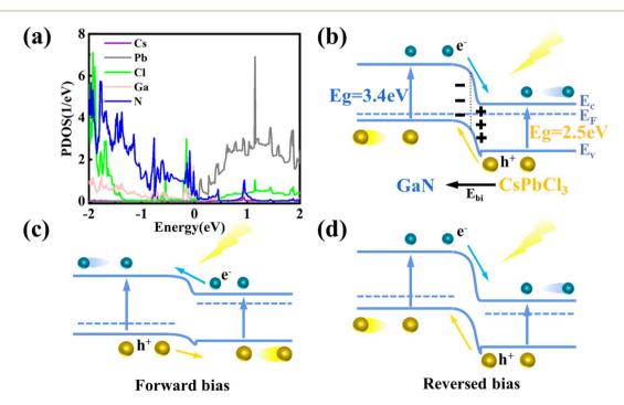
Fig. 5 (a) PDOS of the CsPbCl<sub>3</sub>/GaN heterojunction; (b) schematic diagram of the energy band profile of the CsPbCl<sub>3</sub>/GaN heterojunction; schematic diagram of the energy band profile under (c) forward bias and (d) reversed bias.
