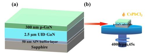
(a) Epitaxial diagram of the p-GaN substrate; (b) spin coating process of CsPbCl<sub>3</sub> nanocrystals.
