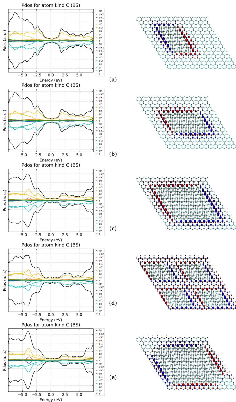
Fig. 8 Comparison of electronic DOS and structures of several G-ane/G-ene systems with island patterns. (a)  $1 \times 64H_{1s}$ . (b)  $1 \times 96H_{1s}$ . (c)  $1 \times 200H_{1s}$ . (d)  $4 \times 50H_{1s}$ . (e)  $1 \times 256H_{1s}$ . Red/blue PDOS correspond to up/down spin.
