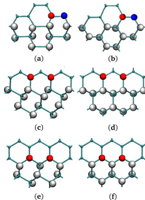
Fig. 4 (a), (c), (e) Chair G-ane isomer at the interface with G-ene. (b), (d), (f) Boat G-ane isomer at the interface with G-ene. (a), (b) AC, (c), (d) ZZ- $\alpha$ , (e), (f) ZZ- $\beta$  terminations of G-ane domain. Two carbon atoms belonging to the nearest neighbor row are shown: the red C atoms are part of sublattice A, the blue of the sublattice B. Check Fig. S9 in ESI† for the definition of a row.
