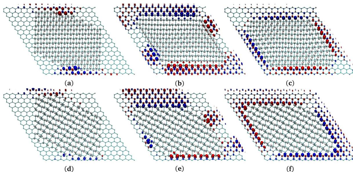
Fig. 5 AC (a and d), ZZ- $\alpha$  (b and c), and ZZ- $\beta$  (e and f) termination of chair (a–c) and boat (d–f) G-ane in G-ene/G-ane interface. Two carbon atoms belonging to the nearest neighbor row are shown: the red C atom is part of sublattice A, the blue of the sublattice B. Red/blue is the  $\pm$  spin density.
