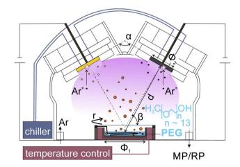
$\alpha = 120^{\circ}$ ,  $\beta = 60^{\circ}$ , d = 110 mm,  $\Phi_1 = 63$  mm  $\Phi_1 = 50$  mm, r = 80 rpm, T = 30 °C, P = 2 Pa
