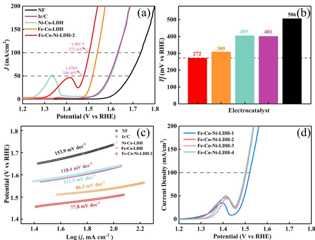
Fig. 6 The OER activity of hollow Fe-Co-Ni-LDH nanocages. (a) Linear sweep voltammetry curves, (b) comparison of OER activity of the samples at a current density of 50 mA cm<sup>-2</sup>, and (c) Tafel plots of the electrocatalysts in 1.0 M KOH solution of NF, Ir/C, Ni-Co-LDH, Fe-Co-LDH and Fe-Co-Ni-LDH. (d) Linear sweep voltammetry curves of Fe-Co-Ni-LDH-1, Fe-Co-Ni-LDH-2, Fe-Co-Ni-LDH-3, and Fe-Co-Ni-LDH-4.
