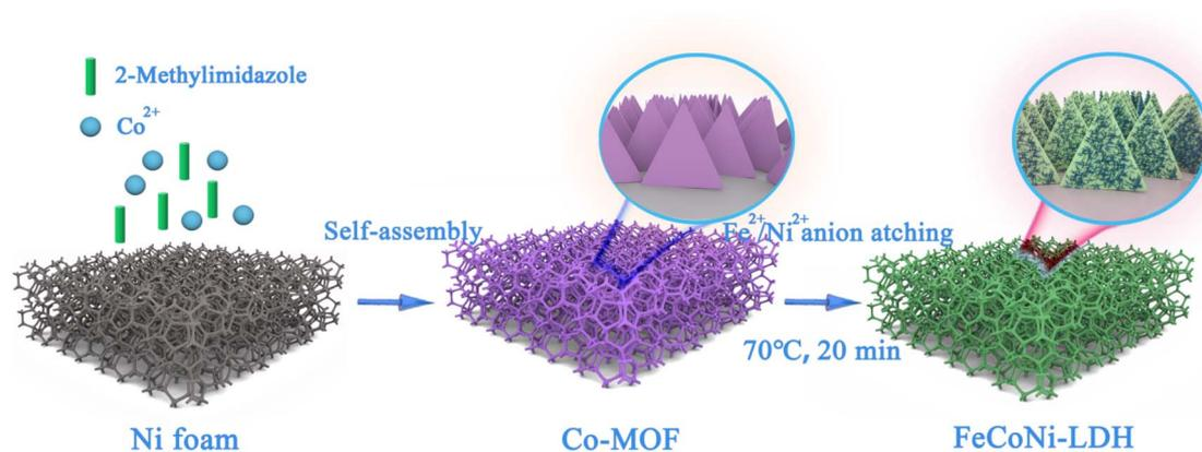
Fig. 1 The preparation of hollow Fe-Co-Ni-LDH nanocages. The uniform hierarchical triangular Fe-Co-Ni-LDH nanocages are prepared via the dication-exchange self-templating strategy.
