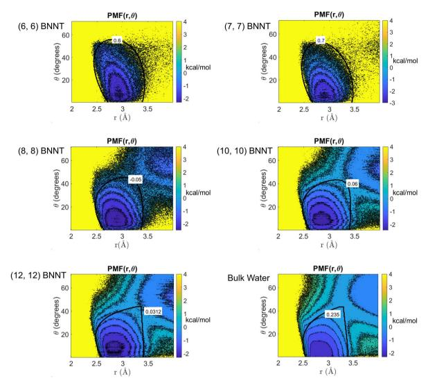
Fig. 2 Two dimensional potentials of mean force (2D PMF) as functions of r and  $\theta$  for water molecules in BNNTs with chiral indices (6, 6), (7, 7), (8, 8), (10, 10) and (12, 12) as well as for water molecules in the bulk. In these figures, the continuous black contour line and the adjacent label (in each figure) indicate the iso-surface separating the HB basin and the corresponding PMF value at this iso-surface, respectively.
