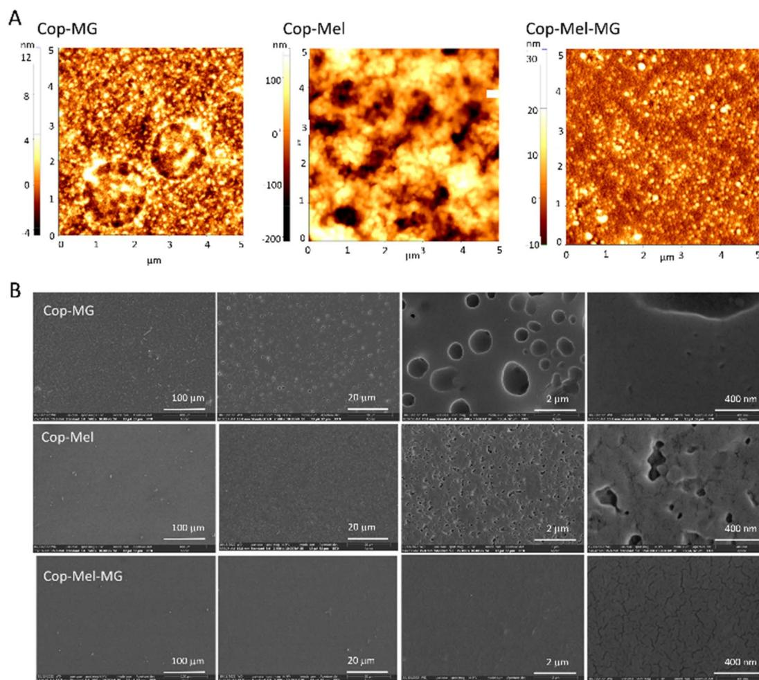
Fig. 1 AFM (A) and SEM (B) images of the topography of the copolymer layers deposited by MAPLE on Si at a laser fluence of  $350 \text{ mJ cm}^{-2}$ , and a number of laser pulses of 72 000 using DMSO as a solvent matrix, in which MG, Mel and both the peptides were incorporated. SEM magnifications are 20 000 $\times$ , 40 000 $\times$  and 150 000 $\times$ .
