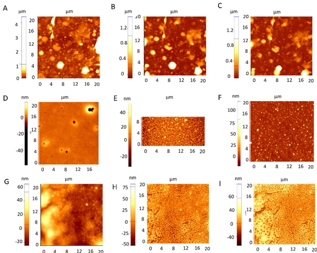
Fig. 4 AFM images of pNIPAM-co-BA-based coatings before (A-Cop, D-Cop-MG, G-Cop-Mel-MG), during immersion in solution with pH 6.4 (B-Cop, E-Cop-MG and H-Cop-Mel-MG) and after drying (C, F and I). The in-liquid scans were made after an immersion time of 30 minutes. For drying, the samples were kept in ambient air for 24 h before scanning again.
