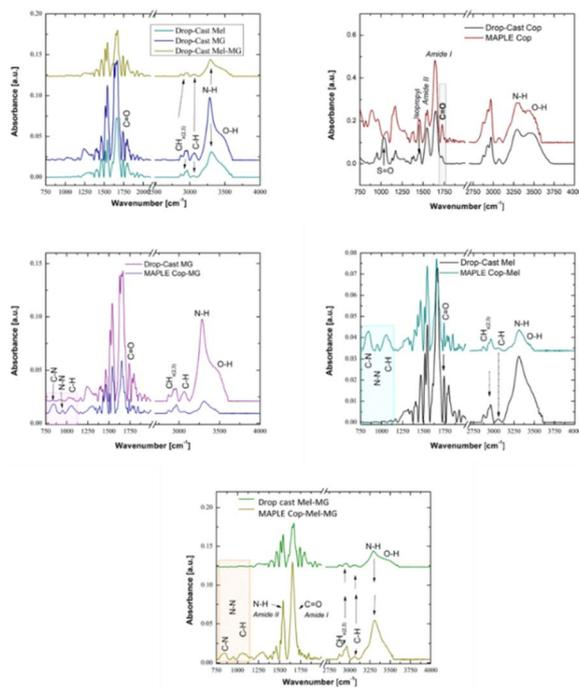
Fig. 3 FTIR spectra of the reference AMPs as separate compounds and combination formula. Comparison MAPLE obtained at 350  $\text{mJ cm}^{-2}$  and DMSO as the solvent vs. the control copolymer layers.
