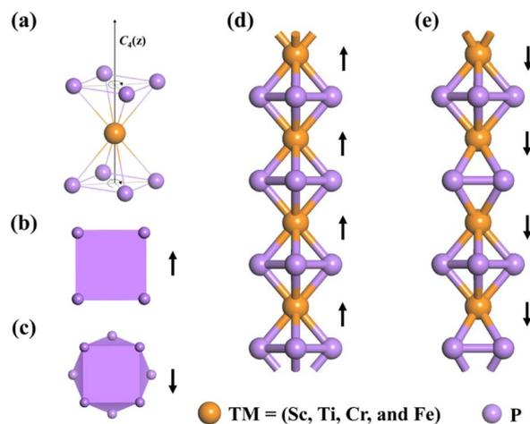
Fig. 1 Models of (a)  $\text{MP}_4$  molecular complex, (b) regular quadrangular prism (Q-type) ligand field, (c) anticube (A-type) ligand field, (d) Q-type  $\text{MP}_4$  nanowire, and (e) A-type  $\text{MP}_4$  nanowire. The "up" and "down" arrows indicate the different stacking models of cyclo- $\text{P}_4$  rings.
