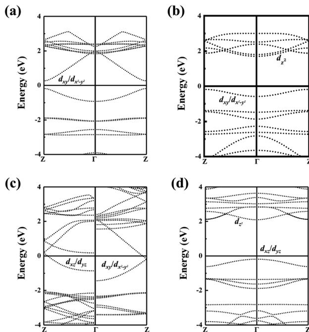
Fig. 2 The electronic band structures for (a)  $ScP_4$ , (b)  $TiP_4$ , (c)  $CrP_4$ , and (d)  $FeP_4$  nanowires at the HSE06 level.
