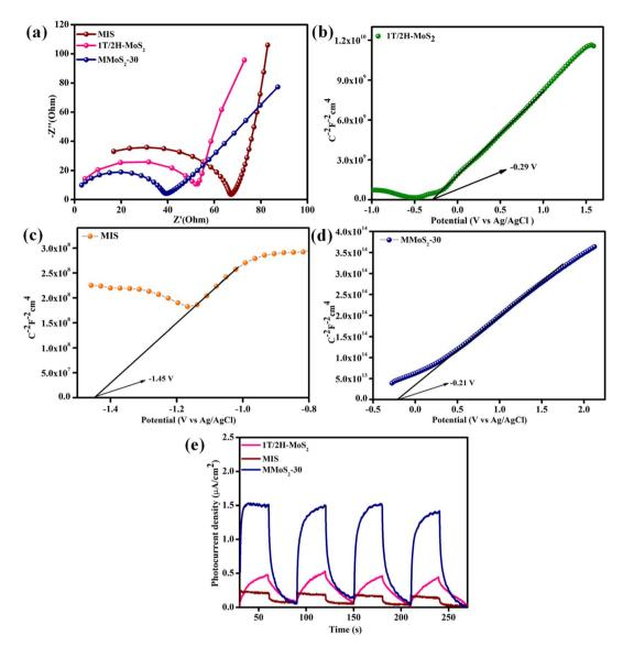
Fig. 4 (a) EIS plot of neat components and the prepared MMoS<sub>2</sub>-30 composite. Mott–Schottky plots of (b) 1T/2H-MoS<sub>2</sub>, (c) MIS and (d) MMoS<sub>2</sub>-30. (e) Transient photocurrent measurement of neat 1T/2H-MoS<sub>2</sub>, MIS, and MMoS<sub>2</sub>-30.
