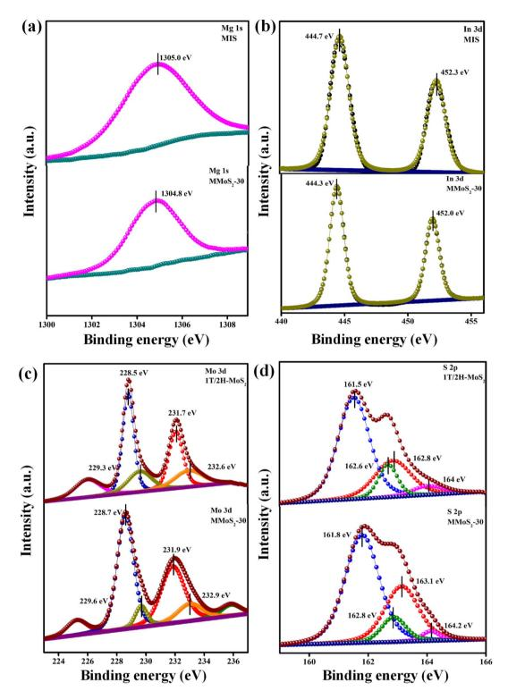
Fig. 2 XPS spectra of neat MIS, 1T/2H-MoS<sub>2</sub> and MMoS<sub>2</sub>-30 composite: (a) Mg 1s, (b) In 3d, (c) Mo 3d, and (d) S 2p.
