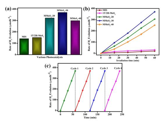
Fig. 5 (a and b) Hydrogen production rate of MIS, 1T/2H-MoS<sub>2</sub>, and synthesized MMoS<sub>2</sub>-x photocatalysts and (c) reusability experiment of the MMoS<sub>2</sub>-30 composite
