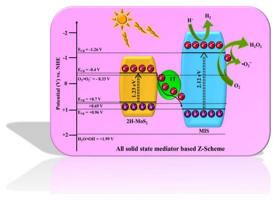
Scheme 2 Schematic representation of the proposed mediator-based Z-scheme charge transfer mechanism of the MMoS<sub>2</sub>-30 photocatalyst for photocatalytic H<sub>2</sub>O<sub>2</sub> and H<sub>2</sub> production under visible light irradiation.
