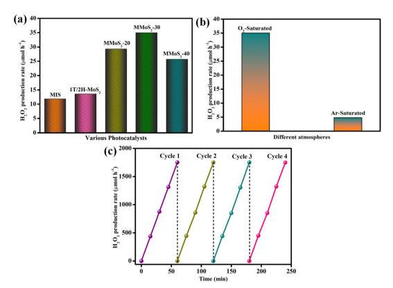
Fig. 6 (a) Rate of photocatalytic H<sub>2</sub>O<sub>2</sub> evolution by neat MIS, 1T/2H-MoS<sub>2</sub> and MMoS<sub>2</sub>-30 photocatalyst. (b) Photocatalytic H<sub>2</sub>O<sub>2</sub> production by  $MMoS_2-30$  composite under different atmospheres and (c) photostability test of the  $MMoS_2-30$  photocatalyst for photocatalytic  $H_2O_2$  evolution.
