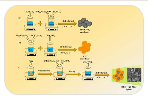
Scheme 1 Synthetic routes for (a) 1T/2H-MoS<sub>2</sub>, (b) MIS and (c) MMoS<sub>2</sub>-x composites via hydrothermal method.
