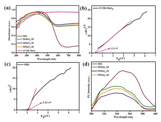
Fig. 3 (a) UV-vis DRS of prepared materials. Band gap energy plots of (b) 1T/2H-MoS<sub>2</sub>, (c) MIS and (d) PL spectra of MIS and MMoS<sub>2</sub>-x composites.
