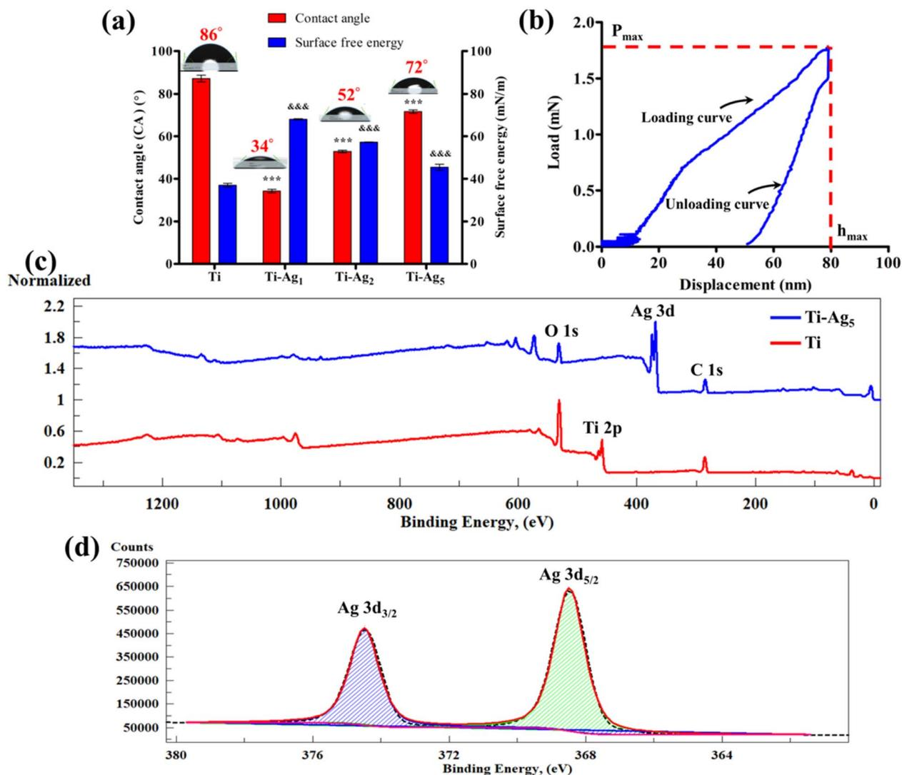
Fig. 2 (a) Assessment of the WCA and SFE of the Ti and Ag-deposited Ti discs. \*\*\* and &#x26; indicate  $p < 0.001$  when compared with Ti. (b) Force-displacement curve of Ti-Ag<sub>5</sub> surface obtained using the nanoindentation technique. (c) XPS survey spectra of Ti (red line) and Ti-Ag<sub>5</sub> (blue line). (d) High-resolution deconvoluted Ag 3d spectra.
