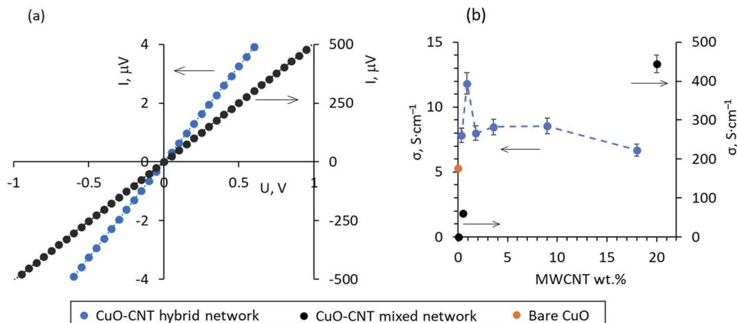
**Fig. 3** (a) Representative current–voltage curves of the CuO–MWCNT hybrid composite with  $\sim 2$  wt% MWCNTs (blue dots, primary axis) and the CuO–MWCNT mixed network with 0.5 wt% MWCNTs (black dots, secondary axis); (b) electrical conductivity of the bare CuO layer (orange dot), CuO–MWCNT hybrid composites (blue dots), and CuO–MWCNT mixed networks (black dots, secondary axis) vs. MWCNT wt% in the network.
