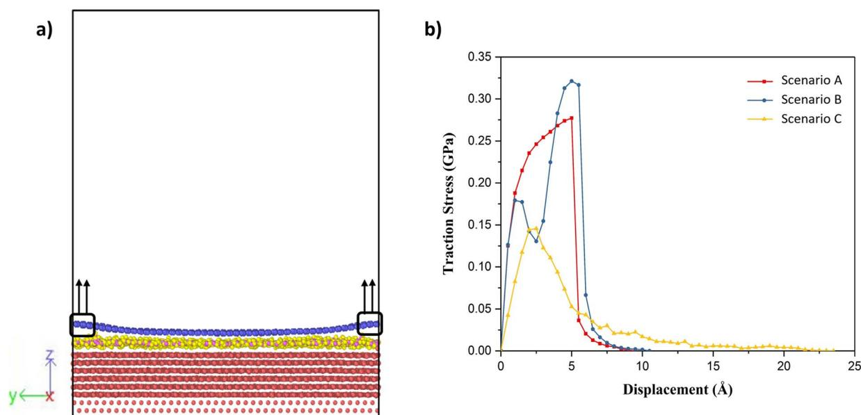
Fig. 4 (a) Schematic of the traction–separation process during simulations, (b) calculated traction–separation curve for each of the scenarios.
