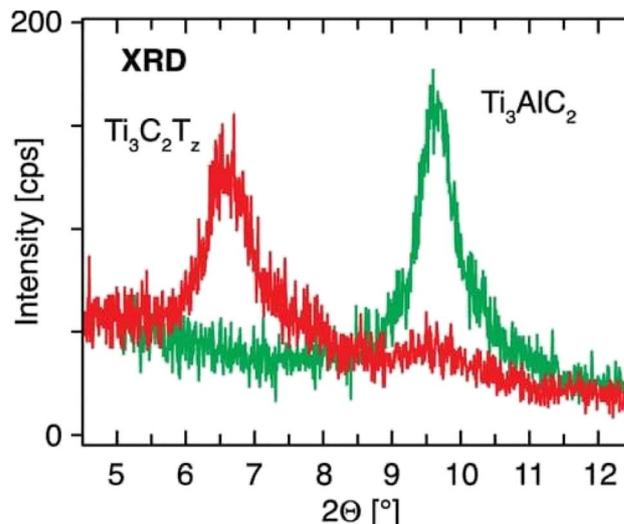
Fig. 7 XRD image of  $\text{Ti}_3\text{AlC}_2$  and  $\text{Ti}_3\text{C}_2\text{T}_x$ . The diffractogram shows the  $\text{Ti}_3\text{AlC}_2$  film at 9.65 and the  $\text{Ti}_3\text{C}_2\text{T}_x$  film at 6.60.<sup>45</sup>
