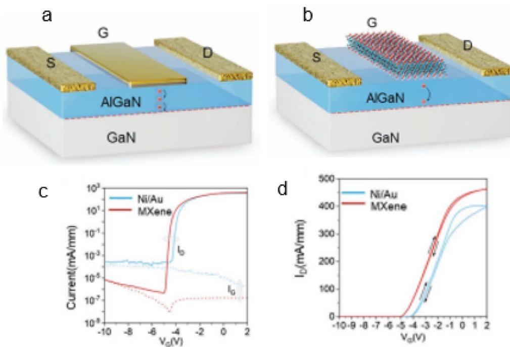
Fig. 18 GaN HEMT schematic diagrams with either  $\text{Ti}_3\text{C}_2\text{T}_x$  or (a) Ni/Au or (b) the gate electrodes. (c) The Ni/Au- and MXene-gate GaN HEMTs'  $I_G$  curves and logarithmic-scale transfer curves. (d) GaN HEMT dual-sweep transfer curves on a linear scale (copyright 2023 John Wiley and Sons).
