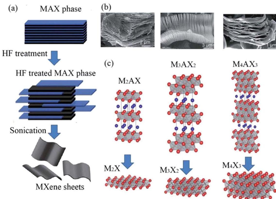
Fig. 1 (a) Three distinct MXene (non-terminated) structures were initially reported:  $M_2X$ ,  $M_3X_2$ , and  $M_4X_3$ . (b) SEM pictures of  $Ti_2AlC$ ,  $Ti_3AlC_2$ , and  $Ti_4AlC_3$  (from right to left) after HF treatment. (c) Illustration of the synthesis of MXenes from MAX phases in a schematic form.
