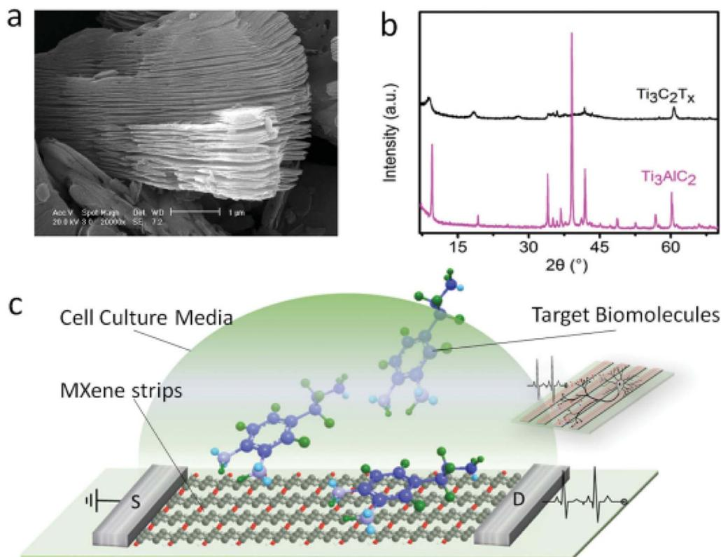
Fig. 17 Characterization of bulk MXenes. (a) SEM image of the multilayer structured MXene. (b) XRD patterns of the transition from  $\text{Ti}_3\text{AlC}_2$  to  $\text{Ti}_3\text{C}_2\text{T}_x$ . (c) Schematic of a biosensing device based on MXene field effect transistors (copyright 2016 John Wiley and Sons).<sup>151</sup>
