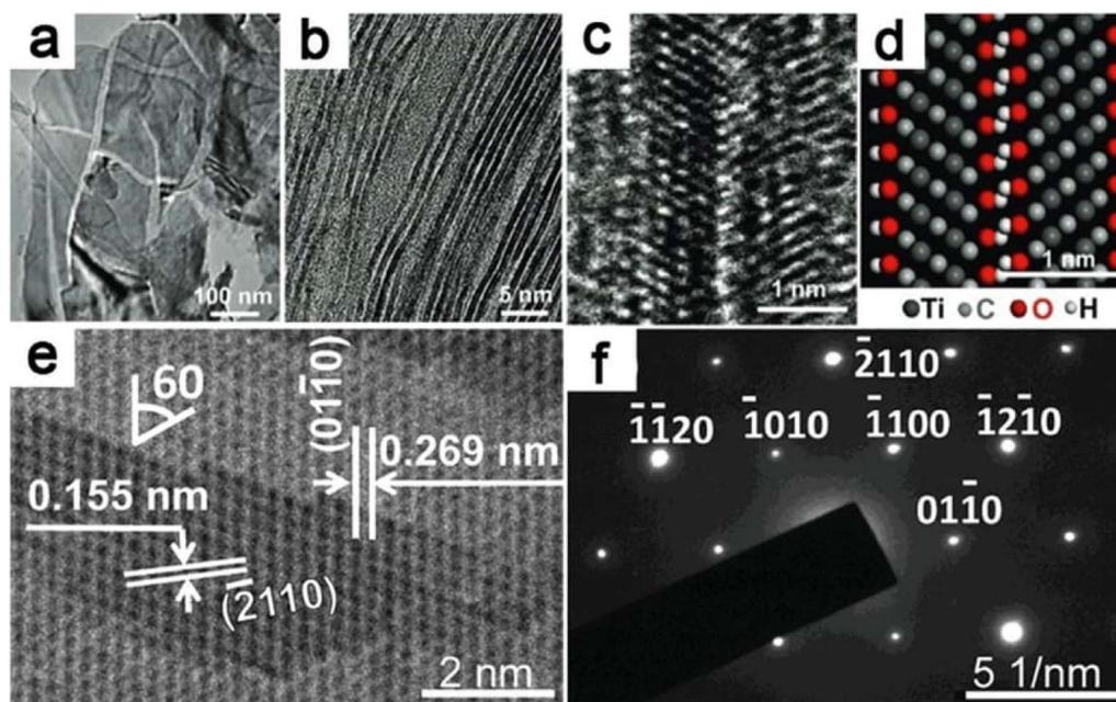
Fig. 10 SAED and TEM imaging of MXenes. (a) A TEM picture of exfoliated Ti–C–O–F 2D nanosheets. (b) MXene sheets with one or two layers. (c) HRTEM picture of bilayer  $\text{Ti}_3\text{C}_2(\text{OH})_x\text{F}_y$  (d) its atomistic model of the layer structure (e) HRTEM image of multilayered MXene and (f) MXene's SAED pattern.<sup>54</sup>
