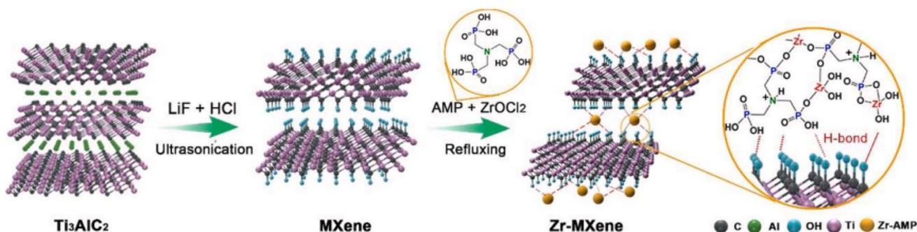
Fig. 3 Scheme for the Zr-MXene preparation.<sup>37</sup>
