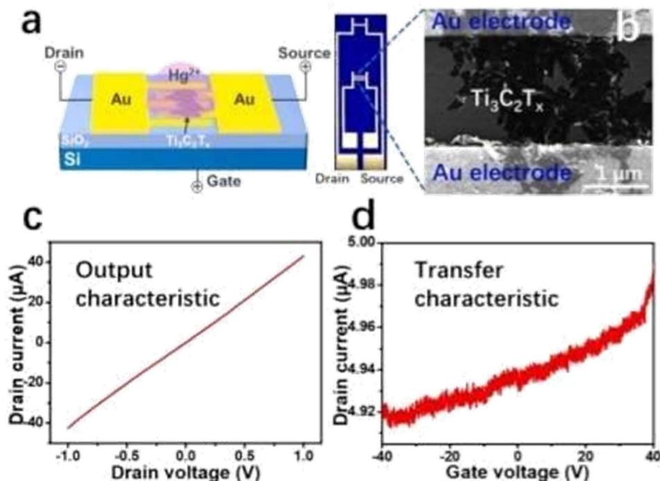
Fig. 11 The  $\text{Ti}_3\text{C}_2\text{T}_x$  FET sensor's schematic structure is shown in (a). (b) A picture of the FET sensor electrodes and a SEM image of the  $\text{Ti}_3\text{C}_2\text{T}_x$  nanosheets joining the nearby gold finger electrodes. (c) A  $\text{Ti}_3\text{C}_2\text{T}_x$  FET device's output characteristics and (d) transfer characteristics.
