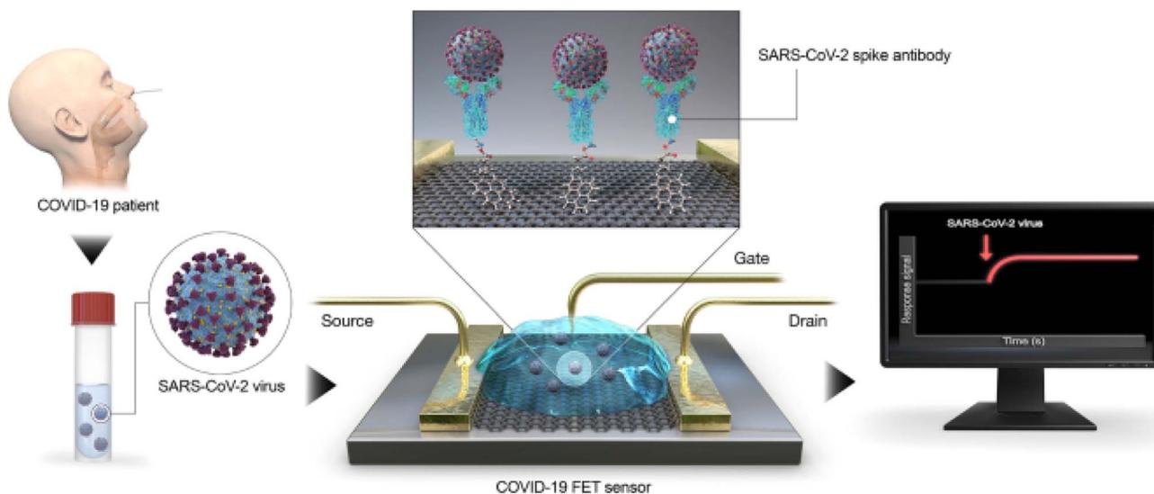
Fig. 15 Diagram showing the steps in the COVID-19 FET sensor functioning. The SARS-CoV-2 spike antibody is attached onto the graphene sheet using the interface molecule 1-pyrenebutyric acid *N*-hydroxysuccinimide ester as a probe linker. Graphene is used as the sensing material.<sup>146</sup>
