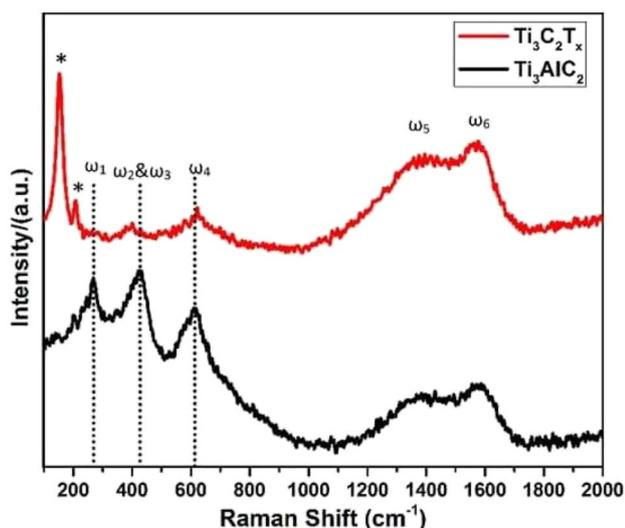
Fig. 5 The Raman spectra exhibit distinctive features for both  $\text{Ti}_3\text{AlC}_2$  MAX powder and  $\text{Ti}_3\text{C}_2\text{T}_x$  MXene. Peaks labeled with "\*" specifically correspond to the out-of-plane vibrations of titanium (Ti) and carbon (C) atoms in the structure.
