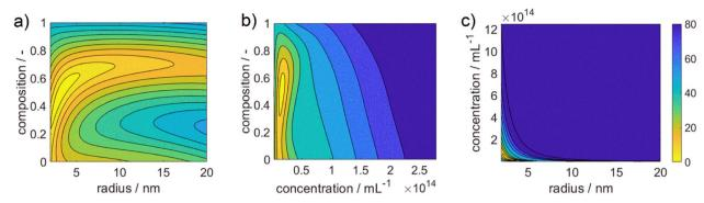
Fig. 3 Plotted cost functional for the color difference of AgAu alloy NPs to the defined color target. The norm of the Euclidean distance in the CIEL\*\*a\*b\*\* space is shown in the color pallet with brighter colors demonstrating smaller distances, i.e., better agreement of color, and darker colors demonstrating larger distances.
