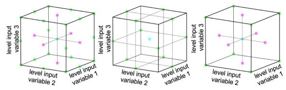
Fig. 1 Comparison of measurement levels around a center point for a full factorial design (left), the Box-Behnken design (middle) and a face centered central composite design (right). Colored dots symbolize measurements.
