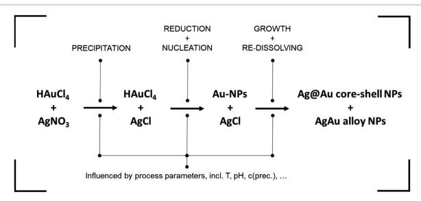
Fig. 4 Schematic formation mechanism of AgAu alloy NPs according to the presented synthesis route. While the steps are shown in subsequent order, in reality all processes run simultaneously with dynamically changing reaction rates and are strongly interconnected.
