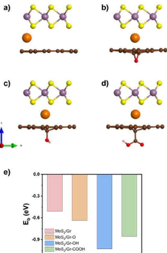
Fig. 1 Side view of optimized (a) MoS<sub>2</sub>/Gr, (b) MoS<sub>2</sub>/Gr-O, (c) MoS<sub>2</sub>/Gr-OH, and (d) MoS<sub>2</sub>/Gr-COOH with Na intercalation (Na marked as orange) and (e) Na binding energy ( $E_b$ ) of each heterogeneous bilayer.
