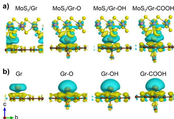
Fig. 2 Charge density difference plot between Na and neighboring (a) heterogeneous bilayers and (b) monolayers (isosurface level: 0.0008 eV Å<sup>-3</sup>). The blue and yellow surface densities represent charge depletion and accumulation, respectively.
