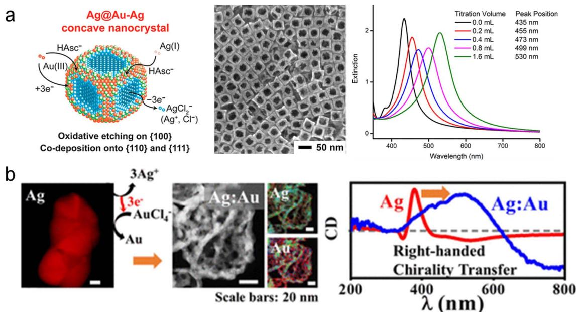
Fig. 6 Multicomponent chiral hybrid nanomaterials prepared by galvanic replacement reactions. (a) AuAg alloy NPs prepared by site-selective GRR between Au ion and Ag NPs.<sup>88</sup> Reproduced from ref. 88 with permission from American Chemical Society, copyright 2018. (b) AuAg chiral alloy NPs prepared by GRR of Au ion and Ag chiral NPs.<sup>89</sup> Reproduced from ref. 89 with permission from American Chemical Society, copyright 2019.
