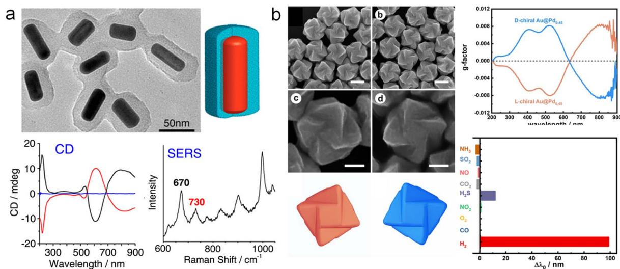
Fig. 11 Chirality sensing using multicomponent chiral plasmon hybrid nanomaterials. (a) Chiral Au NRs@Silica materials for the SERS detection of Cys.<sup>129</sup> Reproduced from ref. 129 with permission from American Chemical Society, copyright 2013. (b) Hydrogen sensing using chiral Au@Pd core-shell NPs.<sup>133</sup> Reproduced from ref. 133 with permission from Wiley VCH, copyright 2023.
