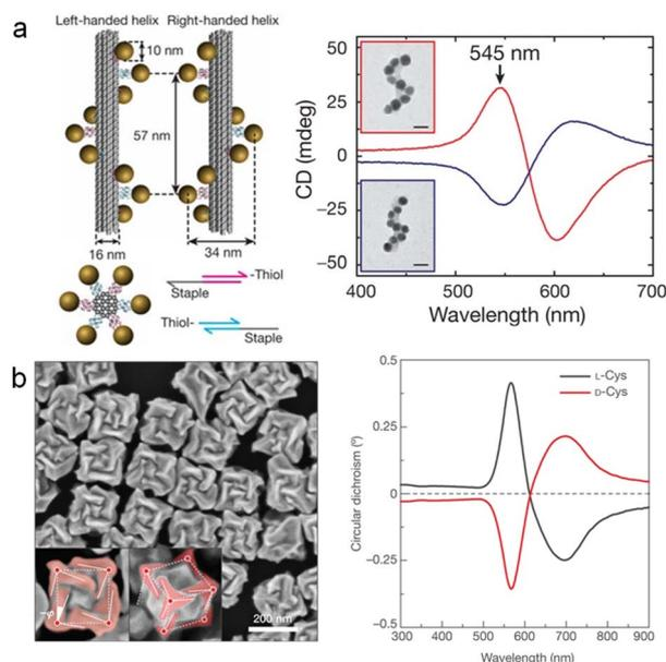
Fig. 2 Typical structures of chiral plasmonic nanomaterials. (a) Chiral assembly of Au NPs templated by DNA origami.<sup>44</sup> Reproduced from ref. 44 with permission from Springer Nature, copyright 2012. (b) Chiral Au NPs with an intrinsic chiral structure prepared by the seed-mediated chiral growth method.<sup>50</sup> Reproduced from ref. 50 with permission from Springer Nature, copyright 2018.
