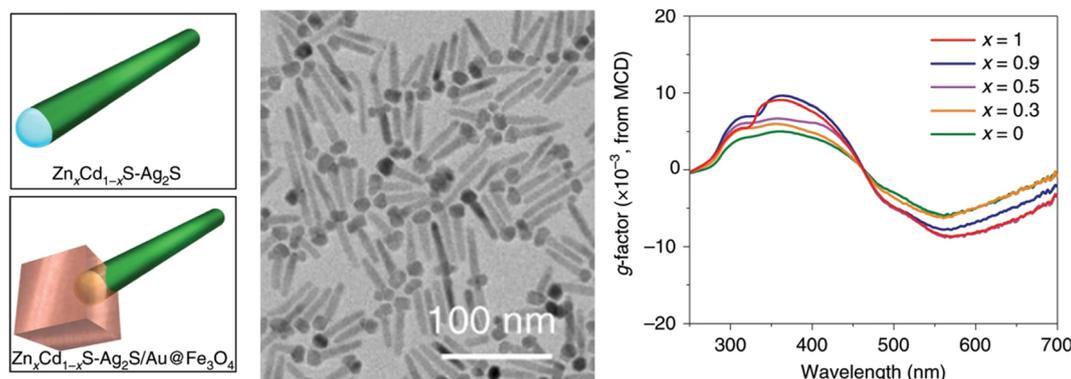
Fig. 9 Multicomponent hybrid materials with magnetically induced chirality. Geometric models, TEM image, and magnetic CD spectra of  $\text{Zn}_x\text{Cd}_{1-x}\text{S-Ag}_2\text{S/Au@Fe}_3\text{O}_4$  hybrid materials.<sup>70</sup> Reproduced from ref. 70 with permission from Springer Nature, copyright 2020.
