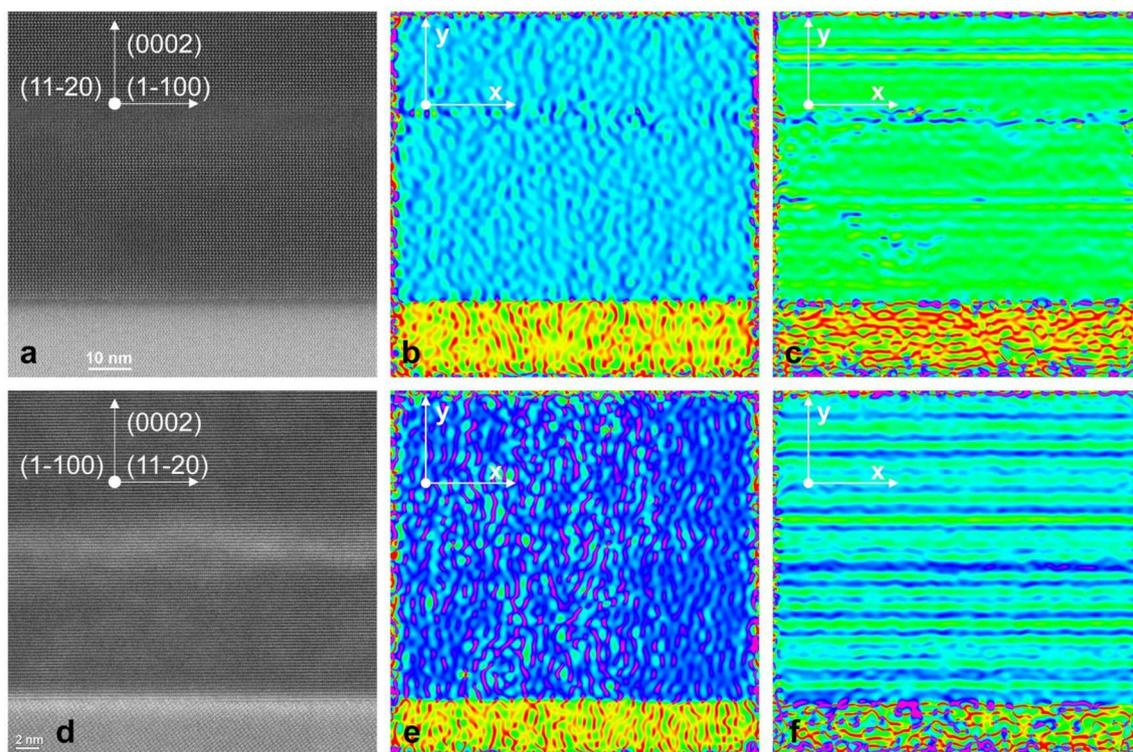
Fig. 4 (a–c) The cross-sectional HR HAADF STEM image along the  $\langle 11-20 \rangle$  direction of the HTA sample near the AlN/sapphire interface and the polarity inversion interface, and the in-plane strain profile  $e_{xx}$  and  $e_{yy}$  GPA images; (d–f) cross-sectional HR HAADF STEM image along the  $\langle 1-100 \rangle$  direction of the HTA sample near the AlN/sapphire interface and polarity inversion interface, and the in-plane strain profile  $e_{xx}$  and  $e_{yy}$  GPA images.
