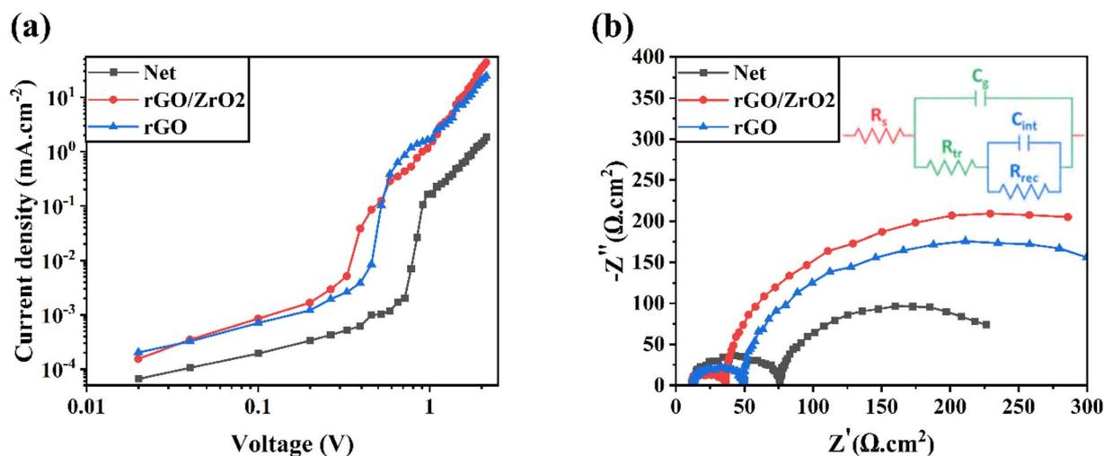
Fig. 7 Electron only and EIS curves of (a) electron-only devices and (b) HTL-free CPSCs based on net, rGO/ZrO<sub>2</sub>, and rGO ETLs.
