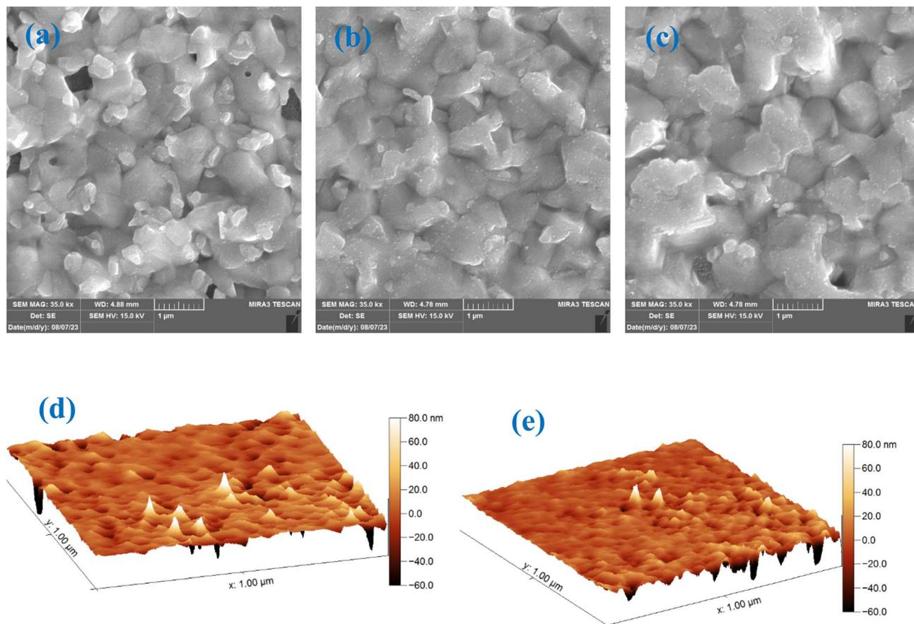
Fig. 6 FESEM images of different perovskite layers fabricated on: (a) Net, (b) rGO/ZrO<sub>2</sub>-, and (c) rGO-doped ETLs. AFM images of (d) Net and (e) rGO/ZrO<sub>2</sub>-doped ETLs.
