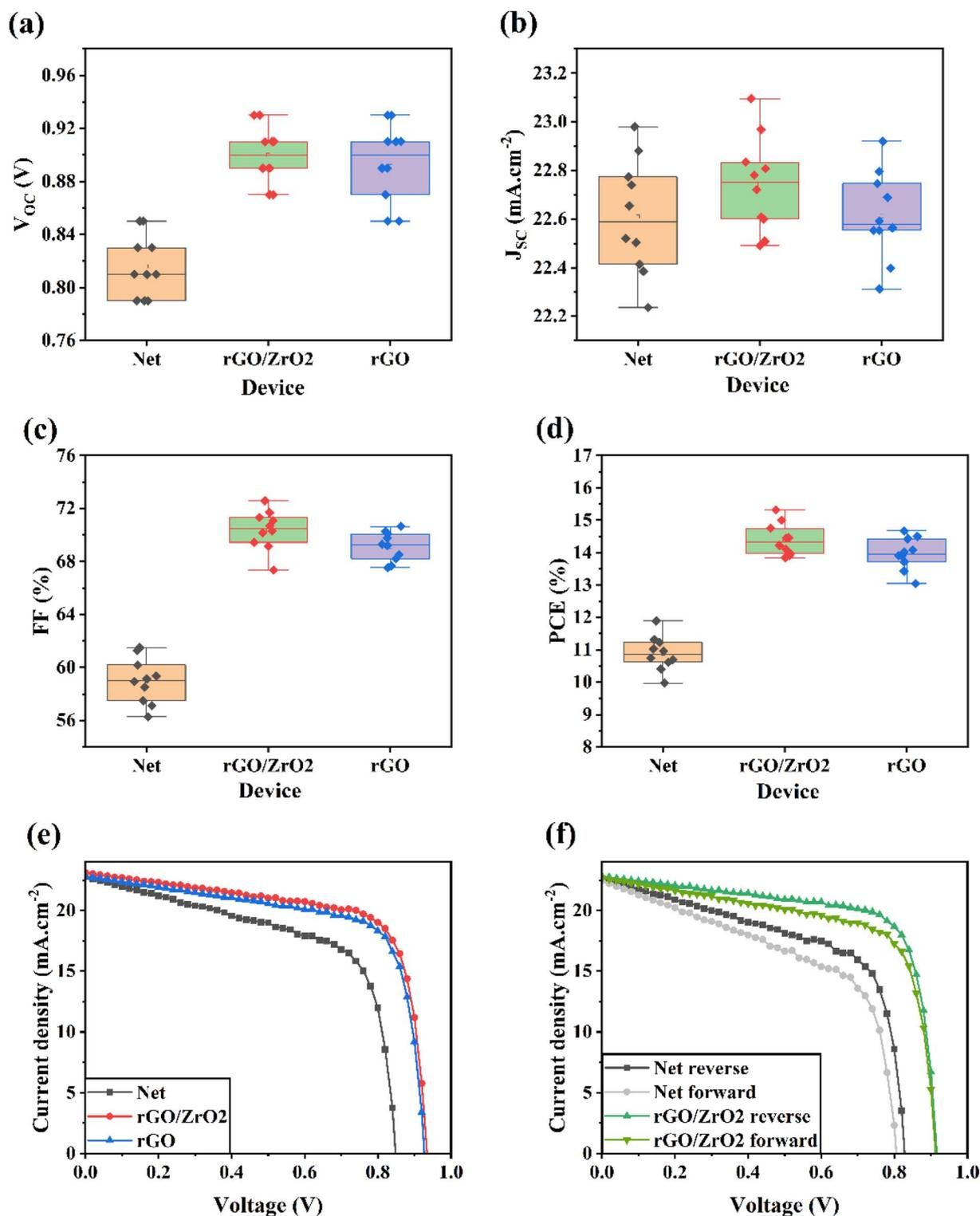
Fig. 2 (a–d) Photovoltaic parameters distributions of HTL-free CPSCs based on different ETLs. (e)  $J-V$  curves of the champion net-, rGO/ZrO<sub>2</sub>-, and rGO-based ETL devices. (f) HI behaviors of the net- and rGO/ZrO<sub>2</sub>-based devices.
