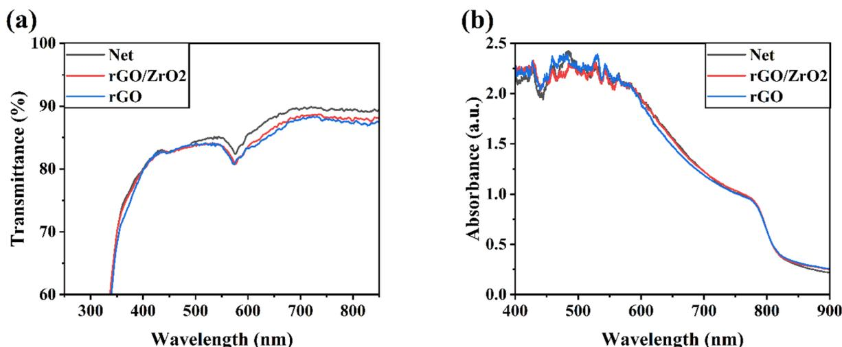
**Fig. 3** (a) Transmittance of different ETLs. (b) Absorbance of perovskites fabricated on different ETLs of net, rGO/ZrO<sub>2</sub>, and rGO.
