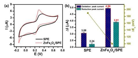
Fig. 4 (a) CV curves and (b) the bar diagram of redox peak currents of 50  $\mu$ M PCM in 0.1 M PBS (pH 5.0). The scan rate of CV is 70 mV s<sup>-1</sup>.
