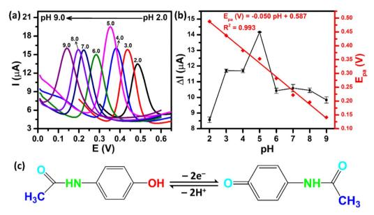
Fig. 8 (a) DPV curves of 250  $\mu$ M PCM at ZnFe<sub>2</sub>O<sub>4</sub>/SPE with different pH values from 2.0 to 9.0; (b) calibration plots of  $\Delta I_{pa}$  and  $E_{pa}$  against pH values: (c) the electrochemical oxidation mechanism of PCM.
