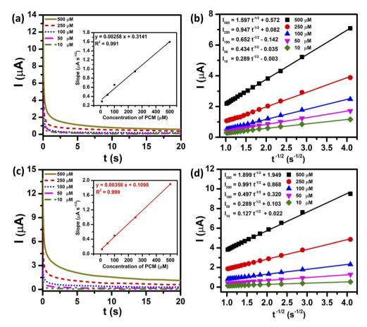
Fig. 6 Chronoamperograms at the bare SPE and ZnFe<sub>2</sub>O<sub>4</sub>/SPE for different concentrations of PCM from 10 to 500  $\mu$ M in 0.1 M PBS (pH 5.0) (a) and (c) and plot of *I* vs.  $t^{-1/2}$  obtained from chronoamperograms (b) and (d). Inset shows the plot of slopes of the resulting straight lines against PCM concentration.
