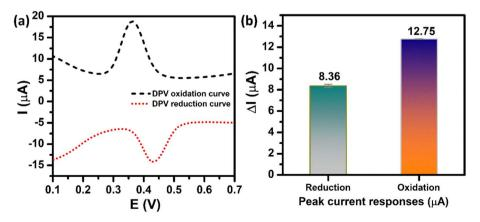
Fig. 7 (a) DPV oxidation/reduction curves and (b) the bar diagram of the oxidation/reduction peak currents of the  $ZnFe_2O_4/SPE$  in 0.1 M PBS (pH 5.0) containing 250 µM PCM.
