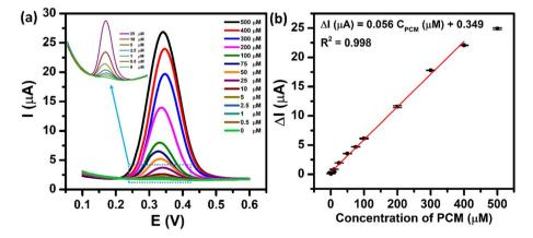
Fig. 9 (a) DPV curves of  $0-500~\mu M$  PCM in 0.1~M PBS (pH 5.0) at the ZnFe<sub>2</sub>O<sub>4</sub>/SPE and (b) the calibration plots of oxidation peak current responses vs. various concentrations of PCM with error bars.
