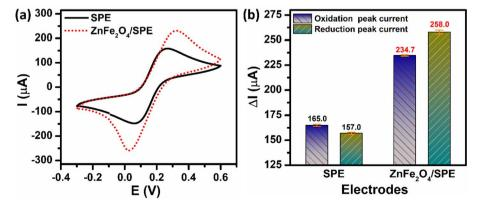
Fig. 2 (a) CV curves and (b) the bar diagram of the oxidation/reduction peak currents of the  $ZnFe_2O_4/SPE$  in 5 mM  $[Fe(CN)_6]^{3-/4-}$  solution containing 0.1 M KCl at a scan rate of 70 mV s<sup>-1</sup>.
