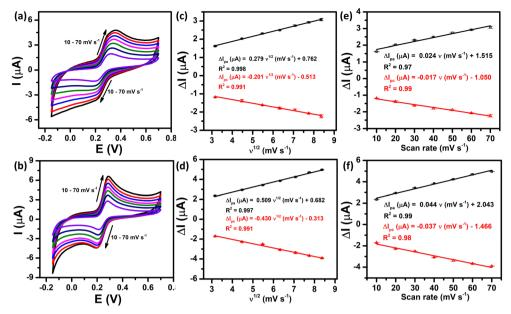
Fig. 5 CV curves recorded at the bare SPE and ZnFe<sub>2</sub>O<sub>4</sub>/SPE in 0.1 M PBS (pH 5.0) containing 50 μM PCM at different scan rates (a) and (b), plots of peak current vs. square root of scan rate (c) and (d), and plots of peak current vs. scan rate (e) and (f), respectively
