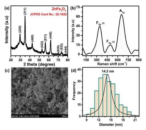
Fig. 1 (a) XRD pattern, (b) Raman spectrum, (c) the FE-SEM image, and (d) the histogram of particle size distribution of ZnFe<sub>2</sub>O<sub>4</sub> NPs.
