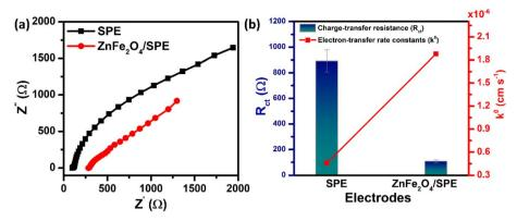
Fig. 3 (a) EIS plots in 5 mM [Fe(CN)<sub>6</sub>]<sup>3-/4-</sup> solution containing 0.1 M KCl for the unmodified and ZnFe<sub>2</sub>O<sub>4</sub>-modified SPE; (b) the bar chart diagram of the charge-transfer resistance ( $R_{ct}$ ) and the heterogeneous electron-transfer rate constant ( $k^0$ ) value of the bare SPE and ZnFe<sub>2</sub>O<sub>4</sub>/SPE.
