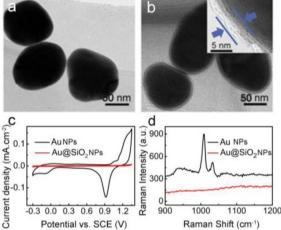
Fig. 1 TEM images for the (a) 80 nm Au NPs and (b) corresponding Au@SiO $_2$  NPs with an external 4–5 nm SiO $_2$  shell. Inset is a TEM image of Ag@SiO $_2$  NPs to show the silica shell. (c) Cyclic voltammograms of Au NPs and Au@SiO $_2$  in 0.5 M H $_2$ SO $_4$  solution, scan rate: 0.1 V s $^{-1}$ . (d) Raman spectrum of pyridine; 0.001 M pyridine on Au and Au@SiO $_2$  on a Si wafer, respectively.
