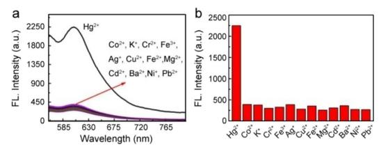
Fig. 4 (a) Fluorescence spectra for the fluorophore-labeled Au@SiO<sub>2</sub> probe in the presence of 1.0 equivalent of Hg<sup>2+</sup>, Cg<sup>2+</sup>, Fe<sup>3+</sup>, Cd<sup>2+</sup>, Fe<sup>2+</sup>, K<sup>+</sup> Cr<sup>2+</sup>, Cu<sup>2+</sup>, Pb<sup>2+</sup>, Mg<sup>2+</sup>, Ag<sup>+</sup>, Ba<sup>2+</sup>, and Ni<sup>2+</sup>. The final concentration of the probe and metal ions are all 0.5 µM. (b) Selectivity of NP sensors plotted in histogram form.
