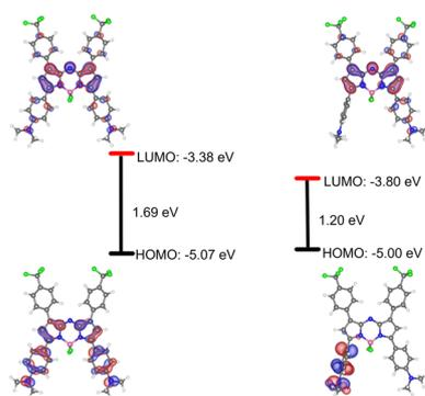
**Fig. 2** Optimized structures and frontier molecular orbitals (HOMO and LUMO) plotted at an electron density value of 0.035 of AZB-CF<sub>3</sub> in ground states (left) and excited states (right) and their corresponding energy gaps ( $\Delta E$  in eV) computed at the B3LYP/6-311G level of theory.
