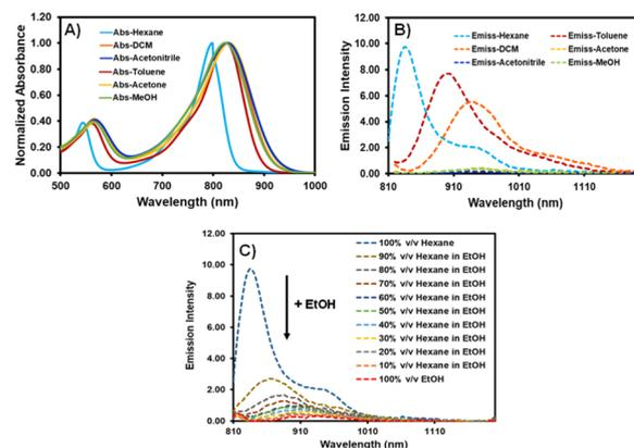
Fig. 1 Absorption (A) and emission (B) spectra of **AZB-CF<sub>3</sub>** in various solvents and (C) emission spectra of **AZB-CF<sub>3</sub>** in hexane–EtOH mixtures (excitation wavelength = 810 nm).
