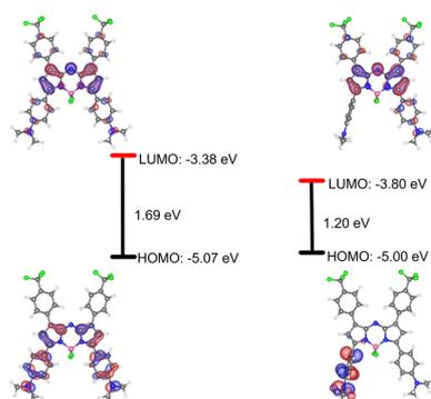
**Fig. 2** Optimized structures and frontier molecular orbitals (HOMO and LUMO) plotted at an electron density value of 0.035 of AZB-CF<sub>3</sub> in ground states (left) and excited states (right) and their corresponding energy gaps ( $\Delta E$  in eV) computed at the B3LYP/6-311G level of theory.
