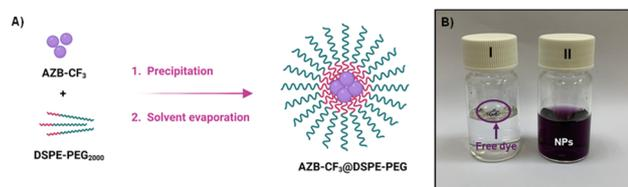
**Fig. 3** (A) Scheme showing the preparation of AZB-CF<sub>3</sub>@DSPE-PEG NPs, (B) vials containing free dye AZB-CF<sub>3</sub> (I) and AZB-CF<sub>3</sub>@DSPE-PEG NPs (II) suspended in PBS.
