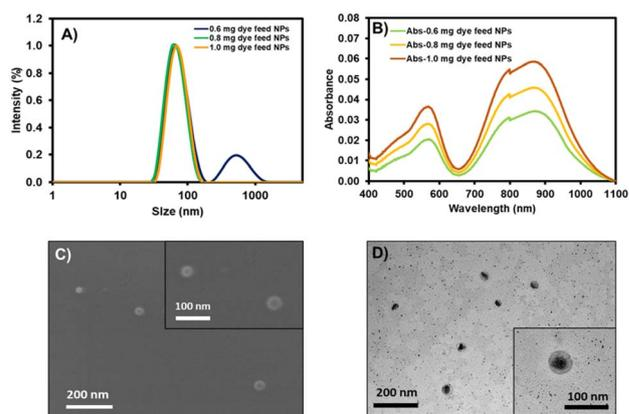
**Fig. 4** (A) Dynamic light scattering (DLS): the intensity-based size distribution of AZB-CF<sub>3</sub>@DSPE-PEG NPs with 0.6 mg, 0.8 mg, and 1.0 mg of dye feed. (B) Absorption spectra of AZB-CF<sub>3</sub>@DSPE-PEG NPs with different amounts of dye feed. (C) Scanning electron microscope (SEM) images and (D) transmission electron microscope (TEM) images of AZB-CF<sub>3</sub>@DSPE-PEG NPs with 1.0 mg dye feed.
