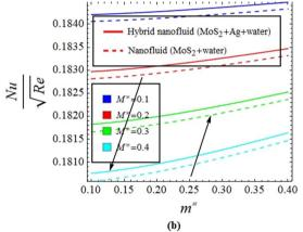
Fig. 4 Impact of  $M^*$  against  $m^*$  on  $C_f\sqrt{Re}$  (a) and  $\frac{Nu}{\sqrt{Re}}$  (b).
