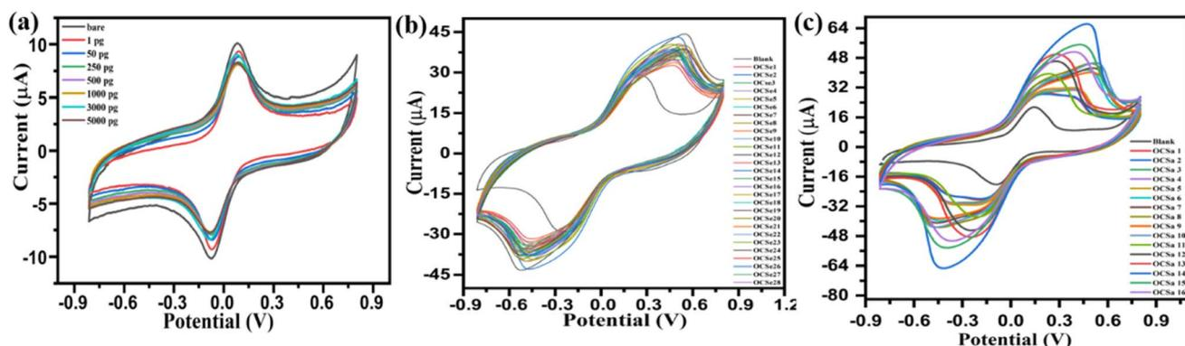
Fig. 9 Cyclic voltammetry studies of the BSA/anti-TP-53/SPE immune-electrode: (a) control plot of BSA/anti-TP-53/SPE vs. TP-53 concentration (0–2000 pg mL<sup>-1</sup>); (b) cancer patient serum sample study using the BSA/anti-TP-53/SPE immune-electrode; (c) cancer patient saliva sample study using the BSA/anti-TP-53/SPE immune-electrode.
