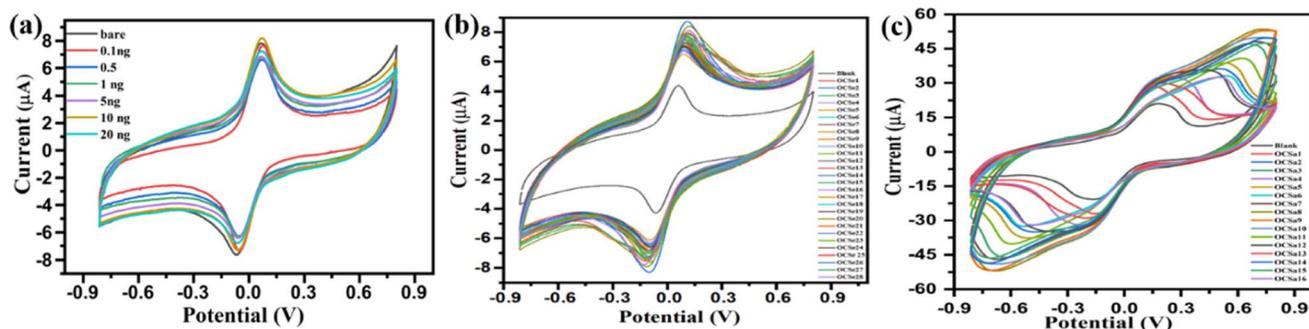
Fig. 7 Cyclic voltammetry studies of the BSA/anti-CYFRA 21-1/SPE immune-electrode: (a) control plot of BSA/anti-CYFRA 21-1/SPE vs. CYFRA 21-1 concentration (0–20 ng mL<sup>-1</sup>); (b) cancer patient serum sample study using the BSA/anti-CYFRA 21-1/SPE immune-electrode; (c) cancer patient saliva sample study using the BSA/anti-CYFRA 21-1/SPE immune-electrode.
