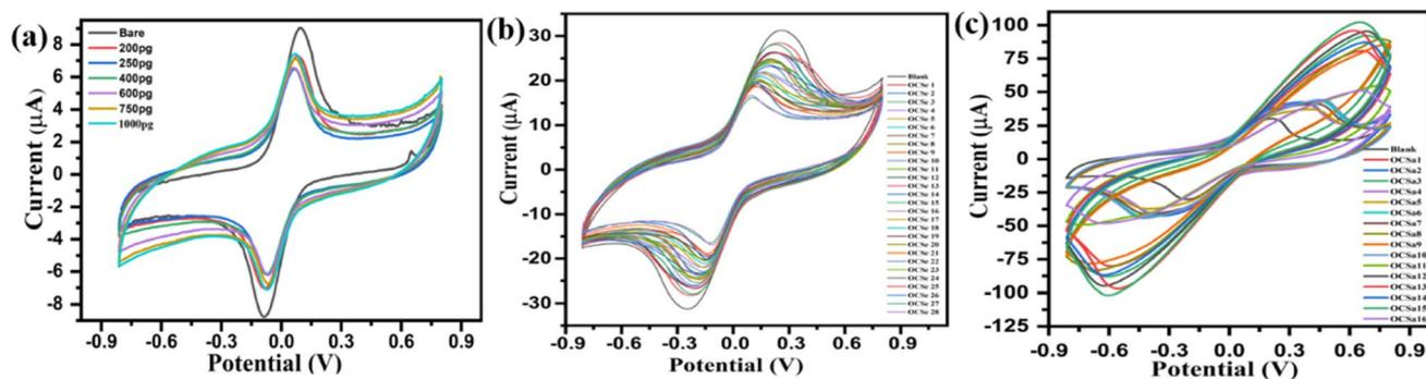
Fig. 8 Cyclic voltammetry studies of the BSA/anti-IL-8/SPE immune-electrode: (a) control plot of BSA/anti-IL-8/SPE vs. IL-8 concentration (0–5000 pg mL<sup>-1</sup>); (b) cancer patient serum sample study using the BSA/anti-IL-8/SPE immune-electrode; (c) cancer patient saliva sample study using the BSA/anti-IL-8/SPE immune-electrode.
