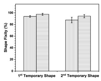
Fig. 12 Shape fixity of (圖) neat and (昌) 3 wt% of GNP reinforced poly(V-fa/urethane) (60/40 wt/wt) nanocomposites for multiple SMP.
