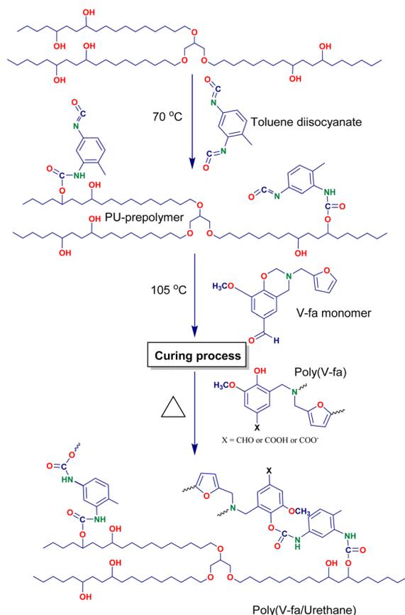
Scheme 2 Preparation of bio-based poly(V-fa/urethane).
