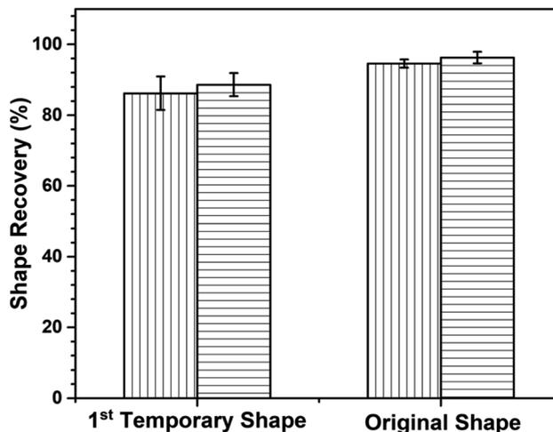
**Fig. 13** Shape recovery of (■) neat and (▨) 3 wt% of GNP reinforced poly(V-fa/urethane) (60/40 wt/wt) composites for multiple SMPs.  $*R_r$  of the 1st temporary shape refers to the performance of the SMP recovered from the 2nd deformed shape state to the 1st deformed shape state.  $*R_r$  of the original shape refers to the performance of the SMP recovered from the 1st deformed shape state to the original shape.
