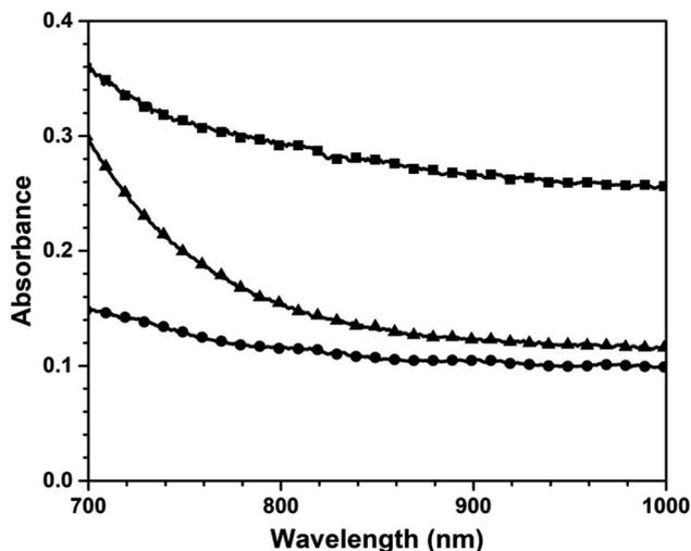
Fig. 10 Vis-NIR absorption spectra of poly(V-fa/urethane) (50/50 wt/wt) with irradiation time: (●) neat poly(V-fa/urethane), (▲) neat poly(V-fa) and (■) 3 wt% of GNP filled poly(V-fa/urethane) nanocomposites.
