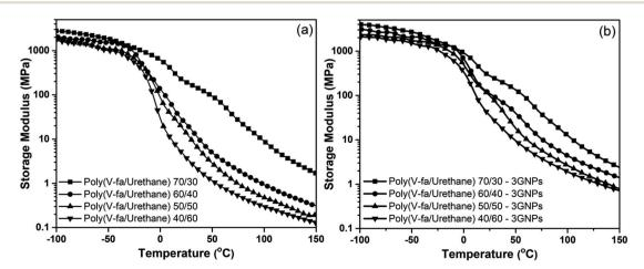
Fig. 4 Storage modulus of (a) neat poly(V-fa/urethane) and (b) poly(V-fa/urethane) nanocomposites filled with 3 wt% GNPs and V-fa/urethane: (■) 70/30, (●) 60/40, (▲) 50/50 and (▼) 40/60.
