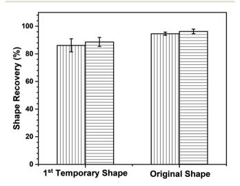
Fig. 13 Shape recovery of ( $\blacksquare$ ) neat and ( $\blacksquare$ ) 3 wt% of GNP reinforced poly(V-fa/urethane) (60/40 wt/wt) composites for multiple SMPs. \* $R_r$  of the 1st temporary shape refers to the performance of the SMP recovered from the 2nd deformed shape state to the 1st deformed shape state. \* $R_r$  of the original shape refers to the performance of the SMP recovered from the 1st deformed shape state to the original shape.
