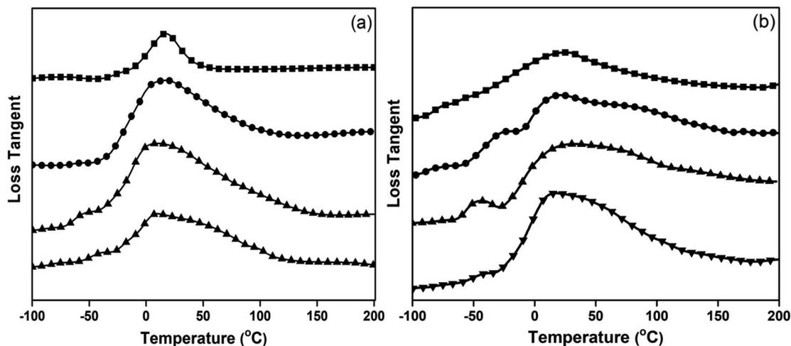
Fig. 5 Loss tangent of (a) neat poly(V-fa/urethane) and (b) poly(V-fa/urethane) nanocomposites filled with 3 wt% GNPs and V-fa/urethane: (■) 70/30, (●) 60/40, (▲) 50/50 and (▼) 40/60.
