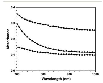
Fig. 10 Vis-NIR absorption spectra of poly(V-fa/urethane) (50/50 wt/ wt) with irradiation time: ( $\bullet$ ) neat poly(V-fa/urethane), ( $\blacktriangle$ ) neat poly(V-fa) and ( $\blacksquare$ ) 3 wt% of GNP filled poly(V-fa/urethane) nanocomposites.
