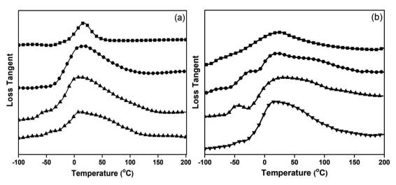
Fig. 5 Loss tangent of (a) neat poly(V-fa/urethane) and (b) poly(V-fa/urethane) nanocomposites filled with 3 wt% GNPs and V-fa/urethane: (■) 70/30, (●) 60/40, (▲) 50/50 and (▼) 40/60.
