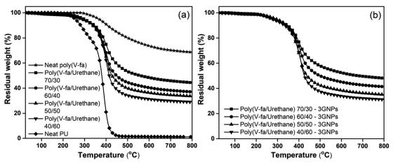
Fig. 3 TGA thermograms of (a) neat poly(V-fa/urethane) and (b) poly(V-fa/urethane) nanocomposites with 3 wt% GNPs and V-fa/urethane: (■) 70/30, (●) 60/40, (▲) 50/50, and (▼) 40/60 composites.
