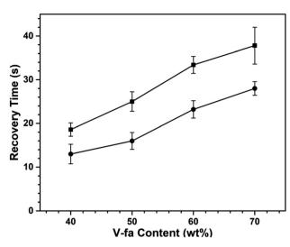
Fig. 8 Recover time under NIR light actuation of poly(V-fa/urethane): (■) neat matrix, and (●) GNP filled nanocomposites.
