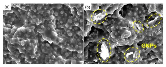
Fig. 16 SEM images of (a) neat poly(V-fa/urethane) and (b) 3 wt% of GNP reinforced poly(V-fa/urethane) (60/40 wt/wt) nanocomposites.
