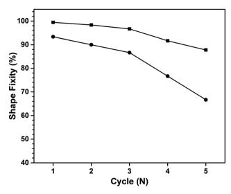
Fig. 14 Shape fixity of 3 wt% of GNP reinforced poly(V-fa/urethane) (60/40 wt/wt) nanocomposites: (■) 1st temporary shape and (●) 2nd temporary shape.
