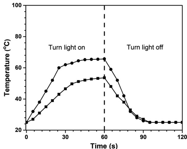
Fig. 9 Variation in temperature of poly(V-fa/urethane) (50/50 wt/wt) with irradiation time: (■) neat poly(V-fa/urethane) and (●) 3 wt% of GNP filled poly(V-fa/urethane) nanocomposites.
