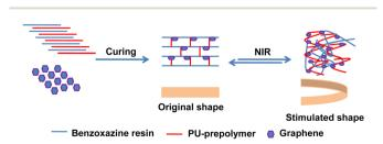
Scheme 3 Shape memory effect of NIR-responsive poly(V-fa/PU) filled with GNPs.
