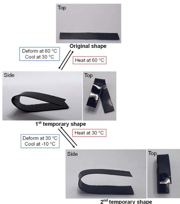
**Fig. 11** Photographs of multiple-shape memory behaviours of poly(V-fa/urethane) (60/40 wt/wt).
