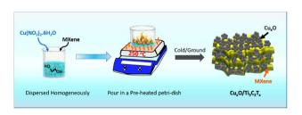
Fig. 1 Schematic illustration of the preparation of the  $\text{Cu}_x\text{O}/\text{Ti}_3\text{C}_2\text{T}_x$  composite.
