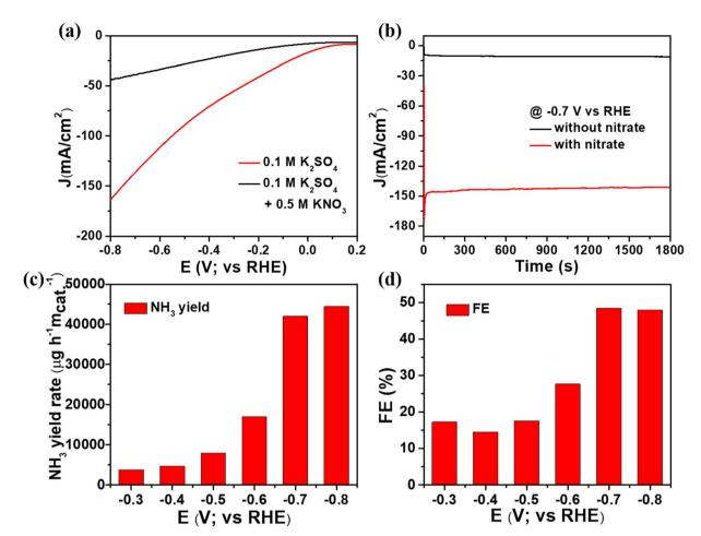
Fig. 4 (a) LSVs curve for  $Cu_xO/Ti_3C_2T_x$  at 10 mV s<sup>-1</sup> with and without nitrate ions in 0.1 M  $K_2SO_4$  electrolyte, (b) chronoamperometric measurements at -0.7 V vs. RHE with and without nitrate ions (c) NH<sub>3</sub> yield and (d) faradaic efficiency for NH<sub>3</sub> production of Cu<sub>x</sub>O/Ti<sub>3</sub>C<sub>2</sub>T<sub>x</sub> catalyst at various potentials
