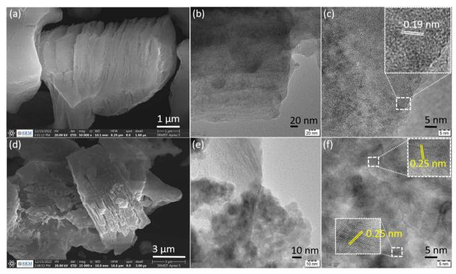
Fig. 3 SEM of (a)  $Ti_3C_2T_x$  and (d)  $Cu_xO/Ti_3C_2T_x$  composite. TEM image of (b and c)  $Ti_3C_2T_x$  and (e and f)  $Cu_xO/Ti_3C_2T_x$  composite.
