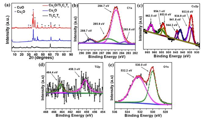
Fig. 2 (a) Comparative XRD patterns of  $Ti_3C_2T_x$ ,  $Cu_xO$  and  $Cu_xO/Ti_3C_2T_x$ . Deconvoluted XPS spectrum for (b) C 1s, (c) Cu 2p, (d) Ti 2p and (e) O 1s of  $Cu_xO/Ti_3C_2T_x$  composite.
