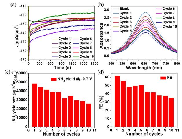
Fig. 5 (a) Chronoamperometric measurements at -0.7 V vs. RHE (b) UV-Vis spectra (c) NH<sub>3</sub> yield and (d) faradaic efficiency for NH<sub>3</sub> production of  $Cu_xO/Ti_3C_2T_x$  catalyst.
