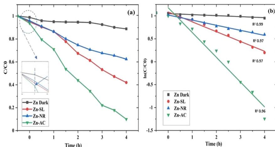
Fig. 11 (a and b) A concentration ( $C/C_0$ ) vs. time plot (a) showing decrease in dye concentration with time for different catalyst systems and (b) a plot of ( $\ln C/C_0$ ) vs. time showing pseudo-first-order kinetics with slope (rate constant " $k$ ") in  $m = -0.04161$  to  $-0.07473$  with  $R^2$  values in the range of 0.95 to 0.99.
