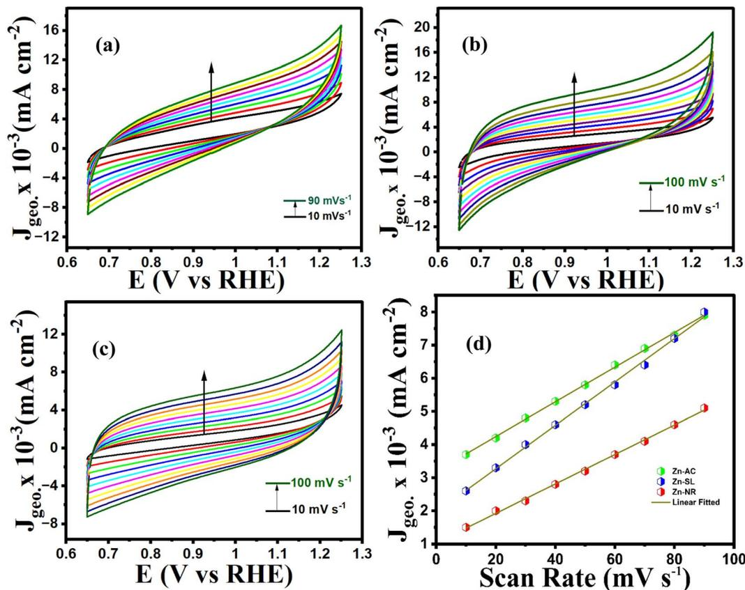
Fig. 14 Cyclic voltammograms (10–100  $\text{mV s}^{-1}$  capacitive region) of (a) Zn-AC, (b) Zn-SL, and (c) Zn-NR catalysts. (d)  $J$  vs. scan rate for the calculation of  $C_{dl}$  (proportional to ECSA) values.
