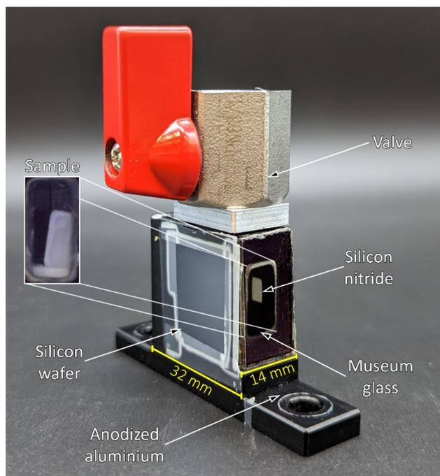
Fig. 5 Photograph of the *in situ* measurement cell consisting of anodized aluminium, a valve on the top, a museum glass in-front, and a silicon wafer and silicon nitride window in direction of the X-ray beam. An exemplary photograph of a gel sample inside the measurement cell is shown on the left side. The scale bars (yellow) of the width and depth are given.
